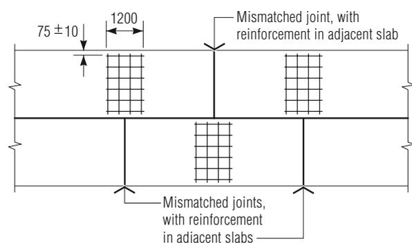
Figure 10.13 Treatment of slabs opposite mismatched joints
