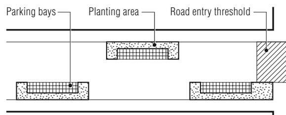
Figure 3.3 Staggered alignment
