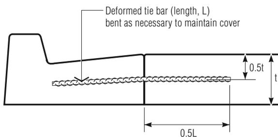
Figure 10.5 Longitudinal joint with kerb and channel
