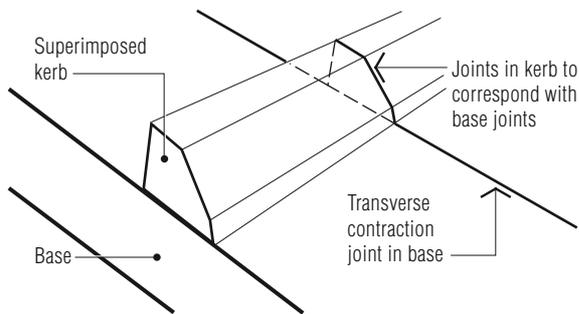
**Figure 11.9** Maintain jointing in super-imposed kerbs and islands
