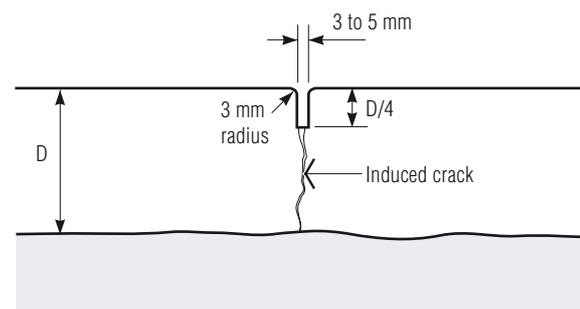
**Figure 11.3** Formed transverse contraction joint
