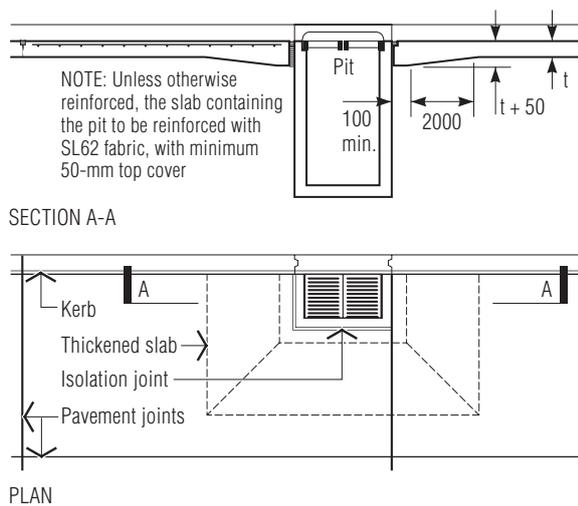
**Figure 10.16** Access holes and pits at pavement edges
