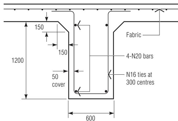
**Figure 10.17** Example of reinforced concrete anchor blocks
