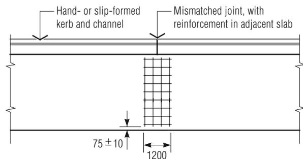
Figure 10.12 Treatment of slab opposite mismatched kerbing joint
