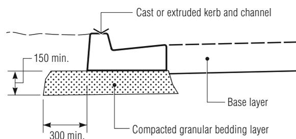
**Figure 11.7** Minimum total thickness of support layer/bedding
