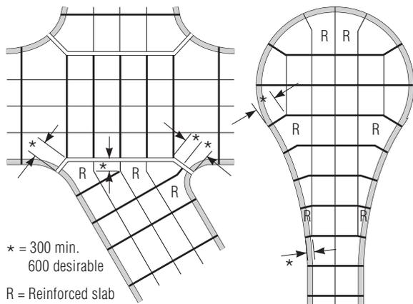
**Figure 10.14** Detailing to avoid acute angles in slabs
