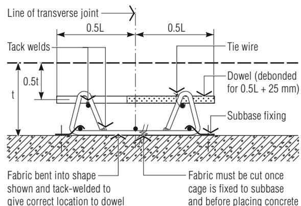
**Figure 10.3 Suggested concrete road pavement dowel assembly**
