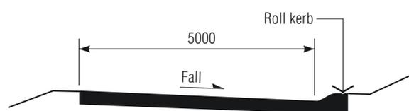
**Figure B1** Typical cross section of pavement
