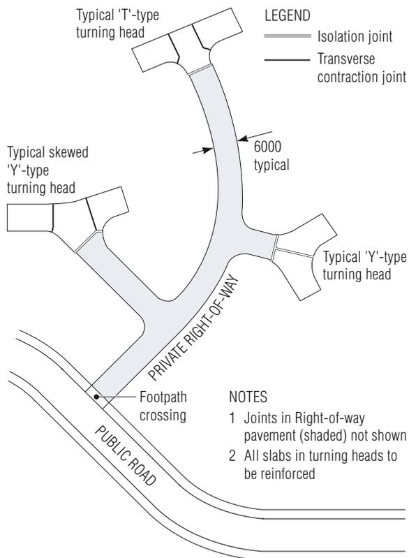
Figure 10.11 Schematic joint layouts for turning areas
