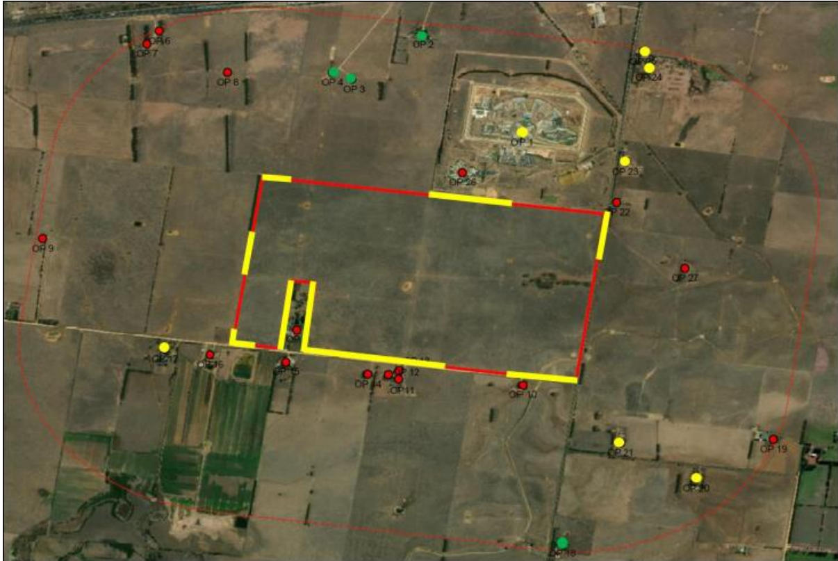
Figure 7-9 - Site layout boundary with receptors and proposed opaque fencing areas (yellow lines)
