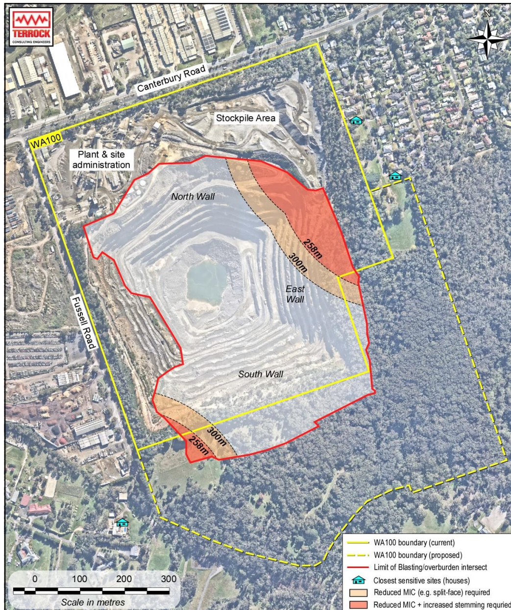
Figure 14 – Extraction areas requiring MIC + stemming height increases for airblast control
