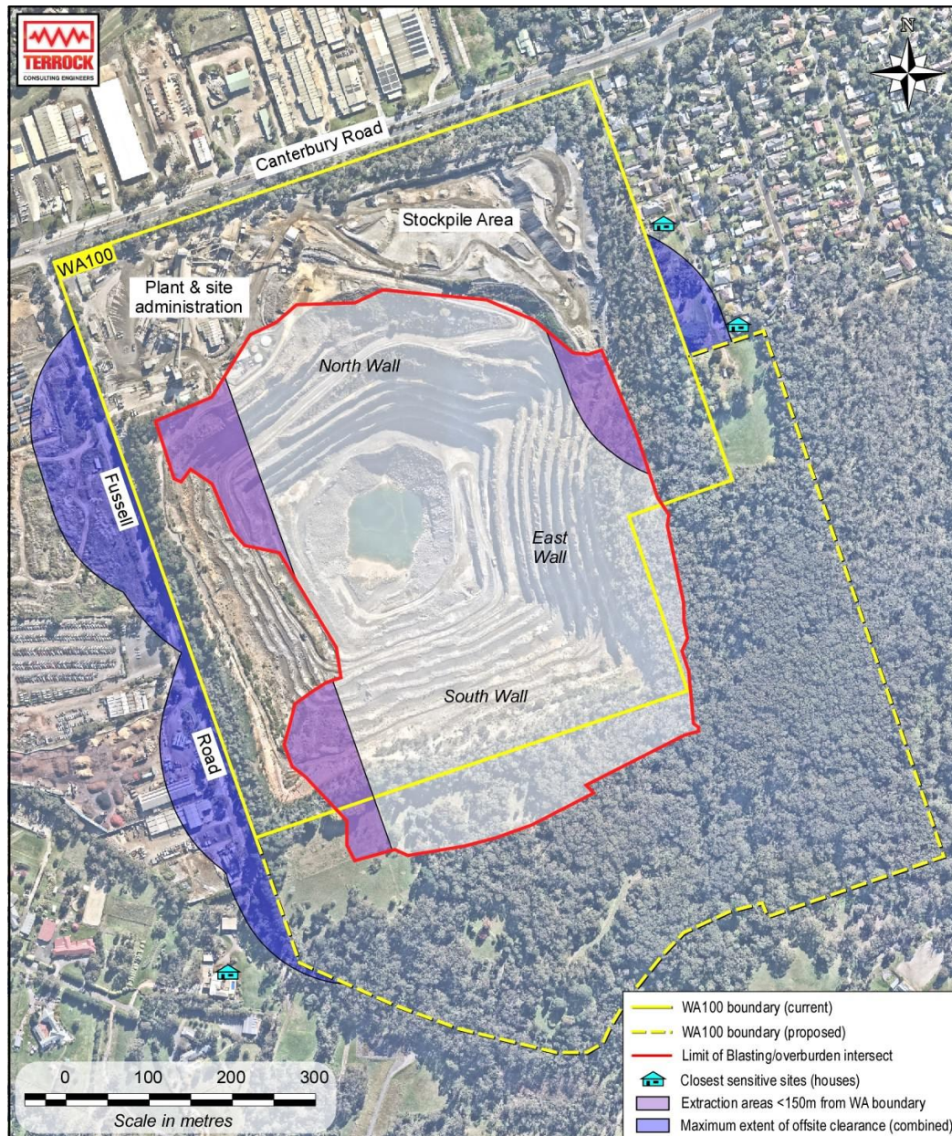
Figure 18 – Maximum (combined) extent of offsite blast clearance (150m), and blast areas <150m from WA100 boundary
