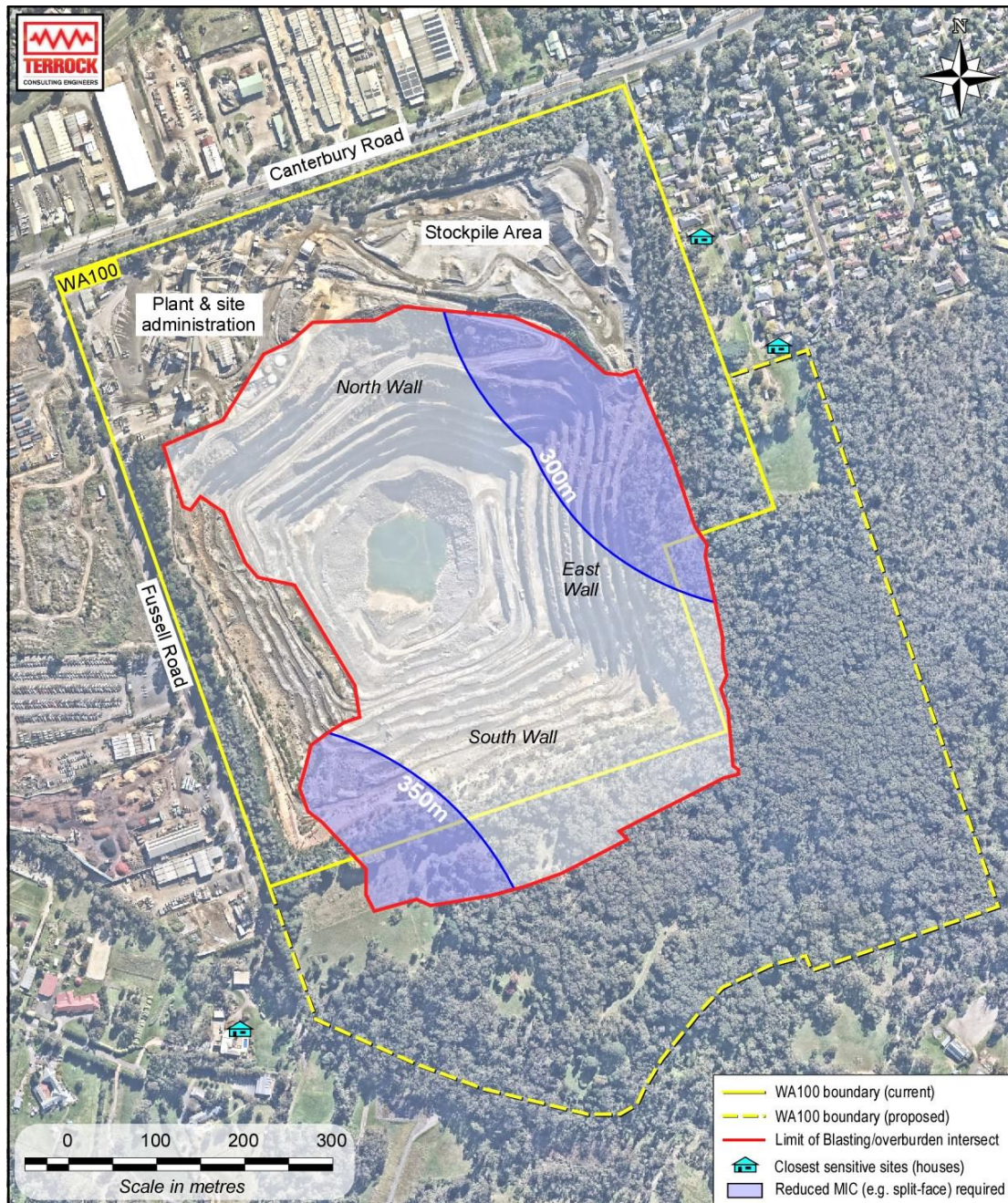
Figure 7 – Extraction areas requiring reduced MIC (<100.2 kg/delay) to maintain PPV levels <5 mm/s
