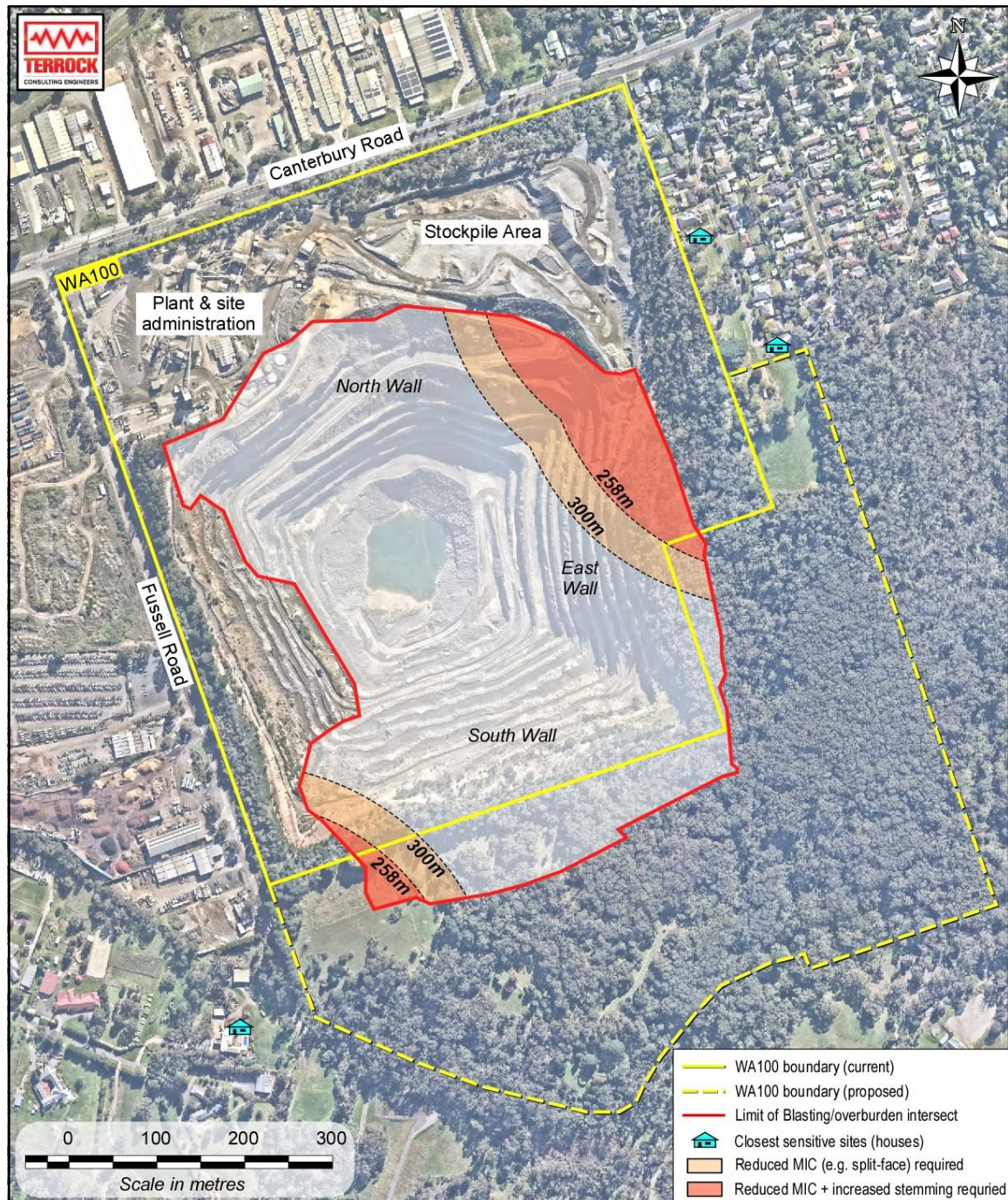
Figure 14 – Extraction areas requiring MIC + stemming height increases for airblast control
