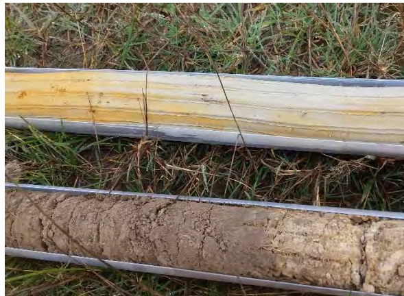
Photo 6: Typical Soil Profile at Depth.
