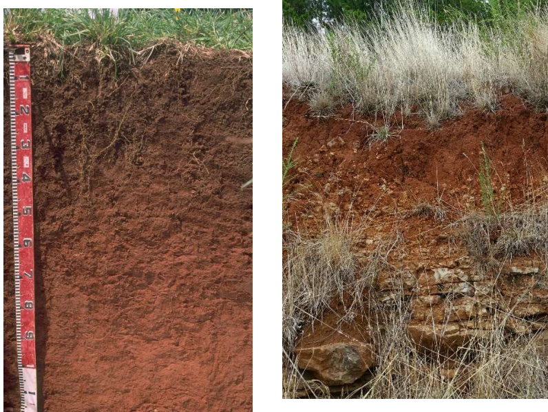
Plate 17. Example Ferrosol soil profiles; on Older Volcanics in West Gippsland (left) and Newer Volcanics near Ballarat (right).
