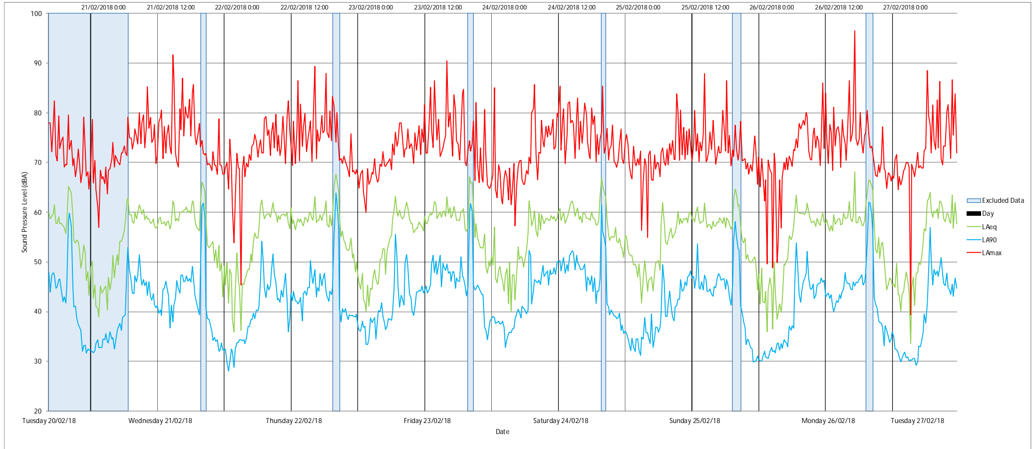
Figure B.7 : Measured sound pressure levels at 350 Stony Point Road, Crib Point. The shaded areas have been removed from the determination of background levels due to excessive road noise and industrial noise sources.
