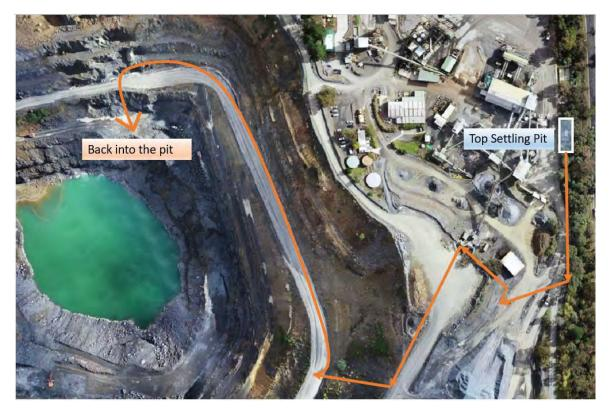
Figure 38 Recycling of water to pit lake
