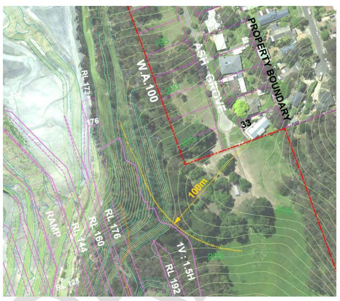
Figure 6 Extraction boundary off-set from residential property boundary above eastern batter
