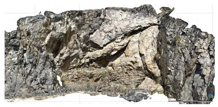
Figure 8 iPad photogrammetry of the southwest shear in the haul road
