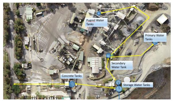
Figure 36 Water reuse and discharge routes
