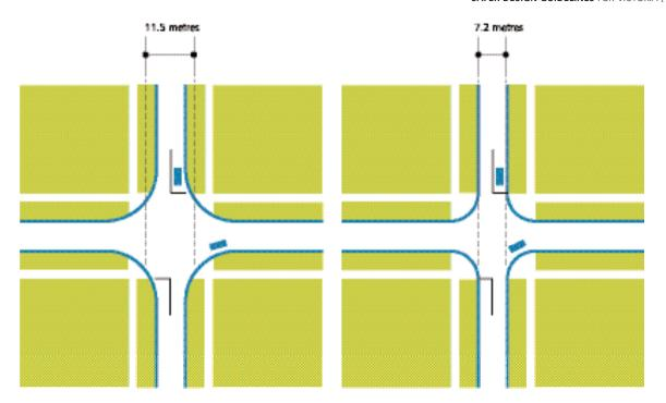
AS THE RADIUS OF THE KERB IS INCREASED, CARS ARE ABLE TO TRAVEL FASTER AND THE DISTANCE PEDESTRIANS HAVE TO CROSS INCREASES MAKING WALKING MORE HAZARDOUS. KEEP KERB RADII TO A MINIMUM AT INTERSECTIONS TO SLOW TRAFFIC AND PROVIDE THE SHORTEST POSSIBLE CROSSING DISTANCE FOR PEDESTRIANS AND OTHER USERS. ENSURE CROSSING POINTS ARE EASILY IDENTIFIED FOR ALL USERS.
