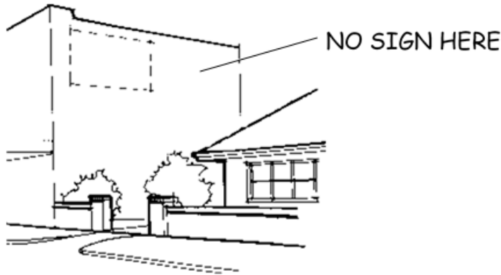
Figure 1 - Location of signs on walls facing residential areas
