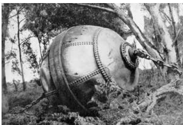
A steel cannon ball for clearing forest 1950s (source: Under Southern Skies [1955])
