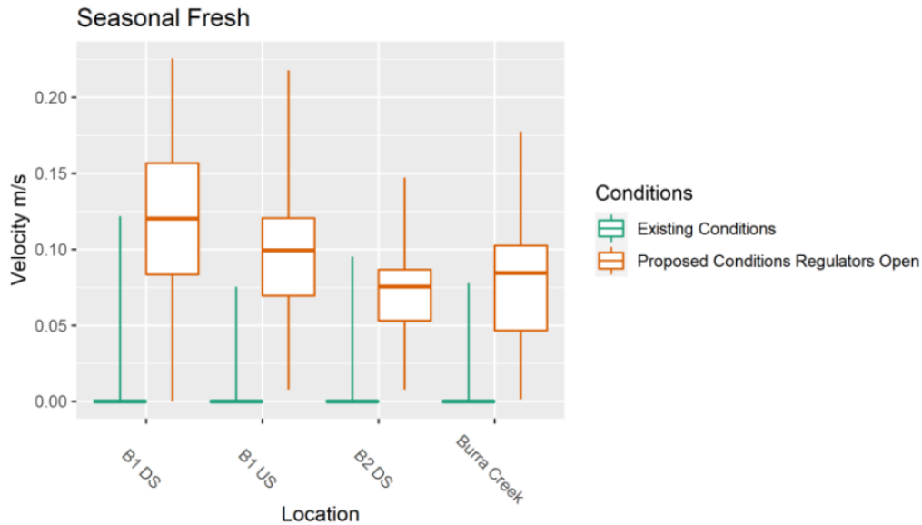
Figure 9 Updated box plots for a Seasonal Fresh equivalent event (around 20,000 ML/day at Swan Hill) – velocity and bed shear stress (Jacobs Burra model)
