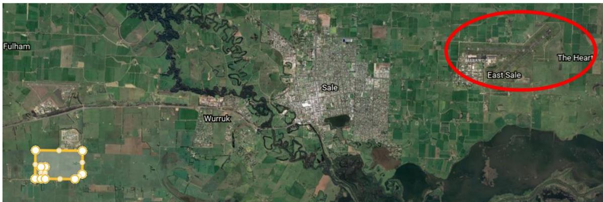
There are two runways at the site. Runway 04 is oriented  $41^{\circ}/221^{\circ}$  from magnetic North whilst Runway 09 is oriented  $086^{\circ}/266^{\circ}$  from magnetic North. The image below details the runways locations at the air base. details the landing and take-off approach direction and ascent/descent angles for the range of flight schools situated at the base.
