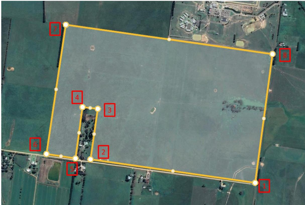
It is important to note that the entire area is not covered with PV panels. To create a more realistic footprint for the purposes of modelling, it is assumed that there is an approximate 15-metre setback from the outside boundaries of the Project with a 15-metre internal setback from the buildings within the site boundary.
