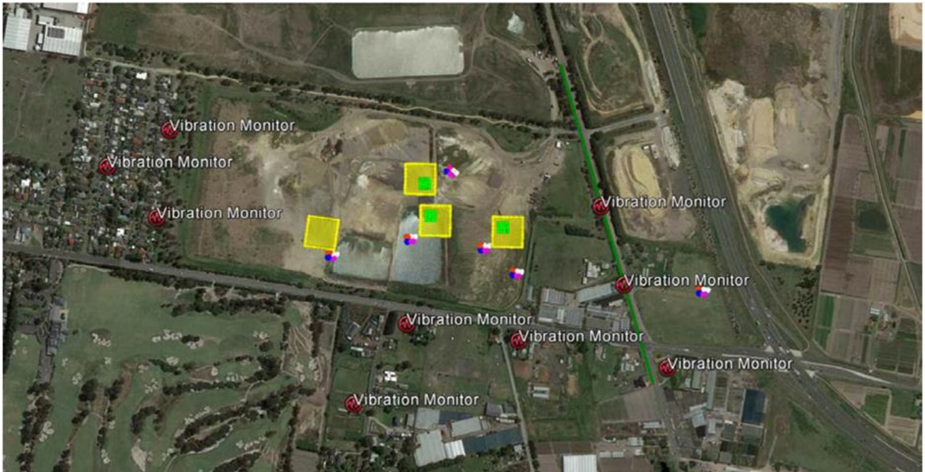
FIGURE 4-6 PROPOSED VIBRATION MONTORING LOCATIONS
