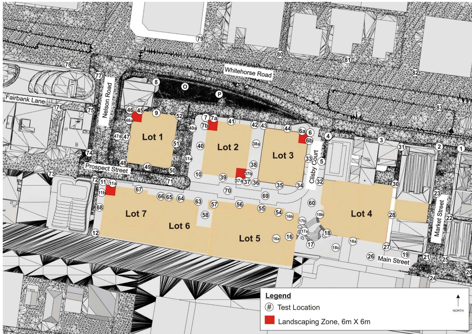
Figure 6 – Ground Level Test Locations in the surrounding streetscapes with wind mitigation strategies.
