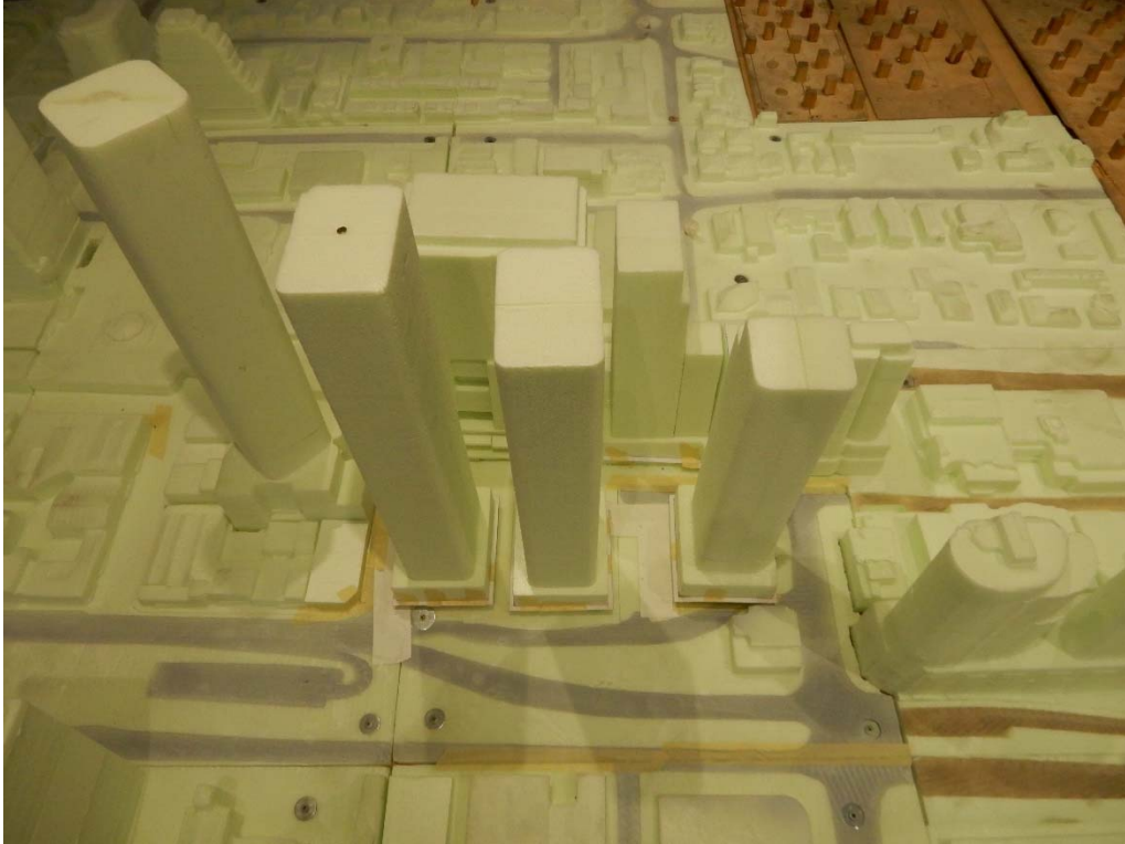
Figure 4 – Close up view from the north of the Box Hill Central North Masterplan Development surrounds in the wind tunnel.
