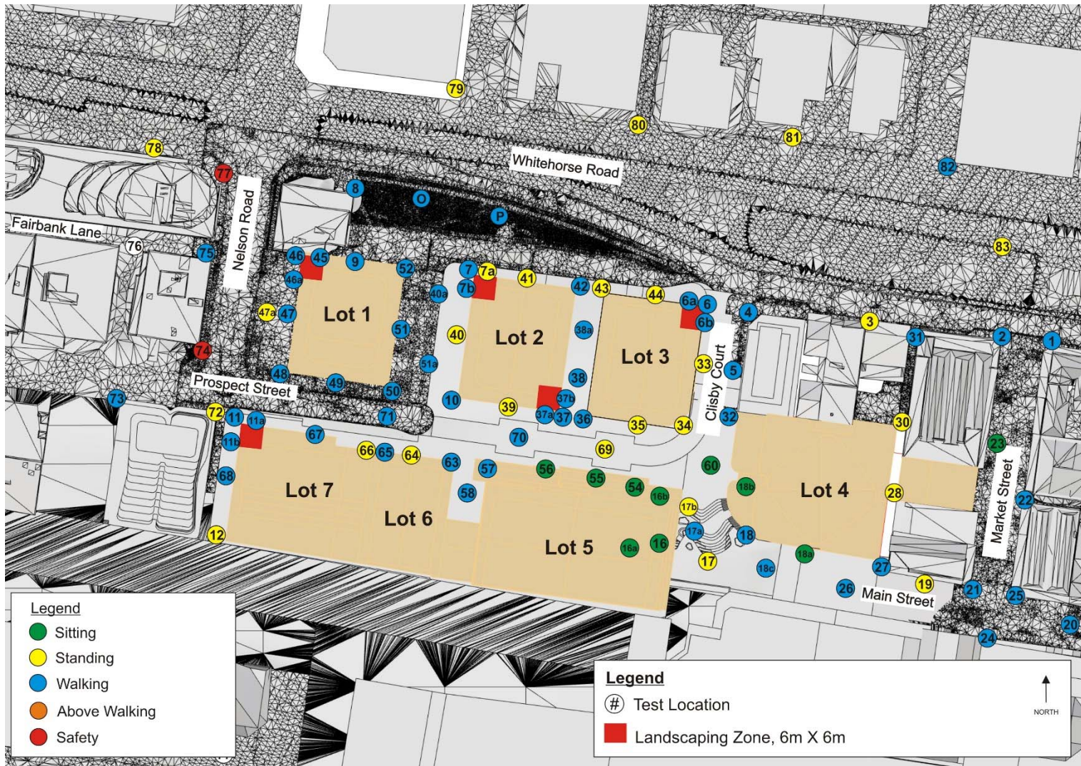
Figure 7b - Summary of wind conditions for the Proposed Configuration of Box Hill Central North Precinct for 360° wind direction.
