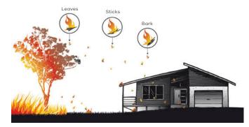
Figure 2 – Ember attack on a structure.
