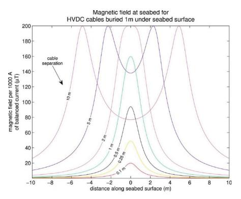
Figure 1: Magnetic field profiles at the seabed surface for a HVDC cable buried 1 m below the seabed. Vertical axis shows the magnetic field per 1,000 amperes of balanced current (in either a bipolar or monopolar with return cable system) (Normandeau et al. 2011)
