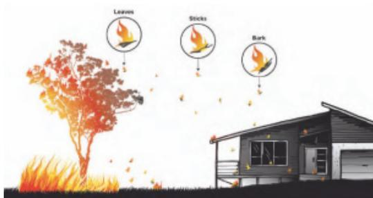
Figure 1 – Ember attack on a structure
