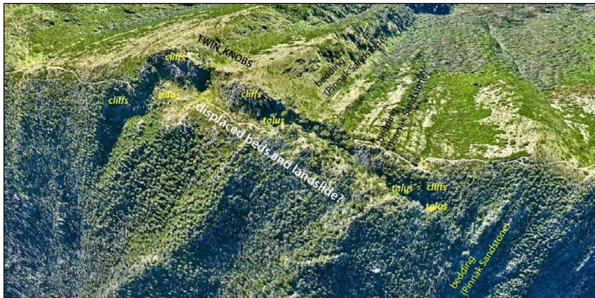
Figure 3-1. Active cliffs and talus slopes of Pinnak Sandstone along the Razorback 500 m south of High Knob. Landslides of varying ages and possible activity are largely confined to the edges and base of basalt at the margins of the Bogong High Plains and in areas above and below parts of Track Sections 06, 07, 10, 11 and 14 with slopes greater than seven degrees. The catchment of Jaithmathang Creek displays a wide range of relict and recent/active slope movements related to a mix of varied geology, steep slopes, rock and groundwater outcrop and relict solifluction materials (Figure 3-2, Figure 3-3).
