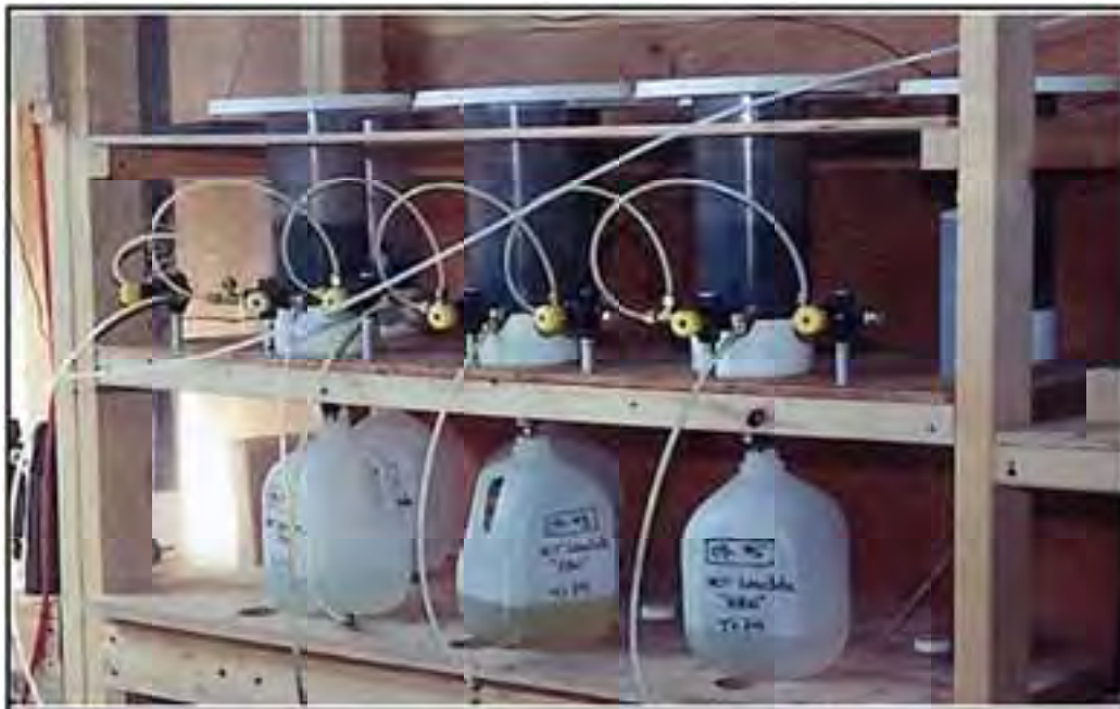
Figure 2: A typical humidity cell test set-up (INAP, 2010)
