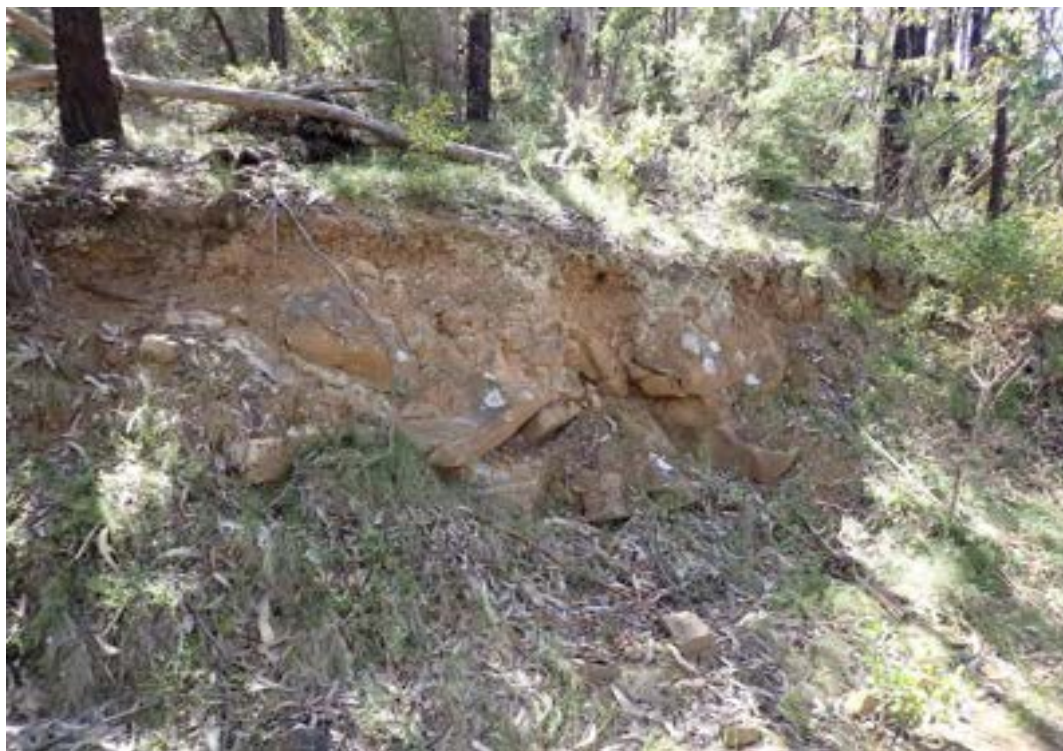
Figure 6: Colluvium overlying distressed sandstone exposed in a cut at the north east abutment
