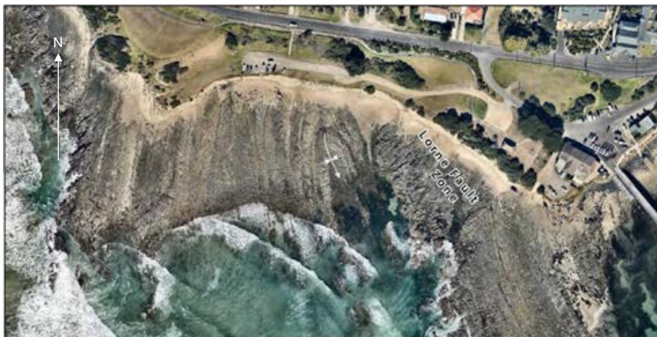
Figure B7: Lorne Fault with a 100 m wide zone of shattered and crushed sandstone and mudstone beds of Eumeralla Formation [A small seaward-plunging synclinal fold west of the fault is probably created by drag on the fault. (Image from Nearmap Dec 2015, structure from Medwell 1988)]
