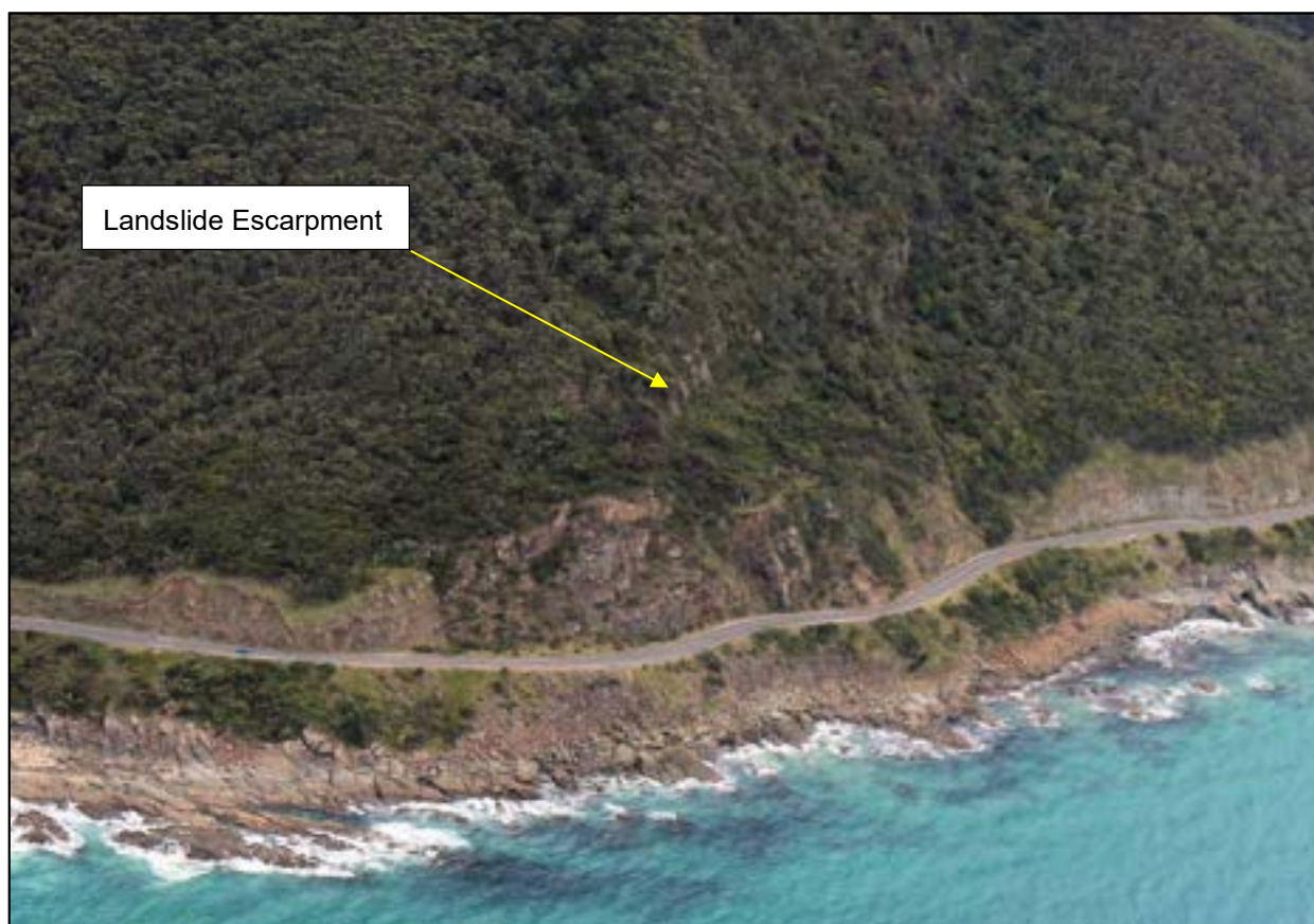
Figure B23: Example of deep-seated landslide in rock at Windy Point (Photo EGS)
