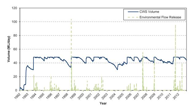
Figure 8: Clean Water Storage (CWS) water volume and modelled environmental release volumes (ML/day) under operating conditions for the 'dry scenario'.
