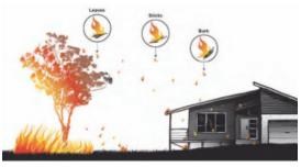
Figure 1 – Ember attack on a structure
