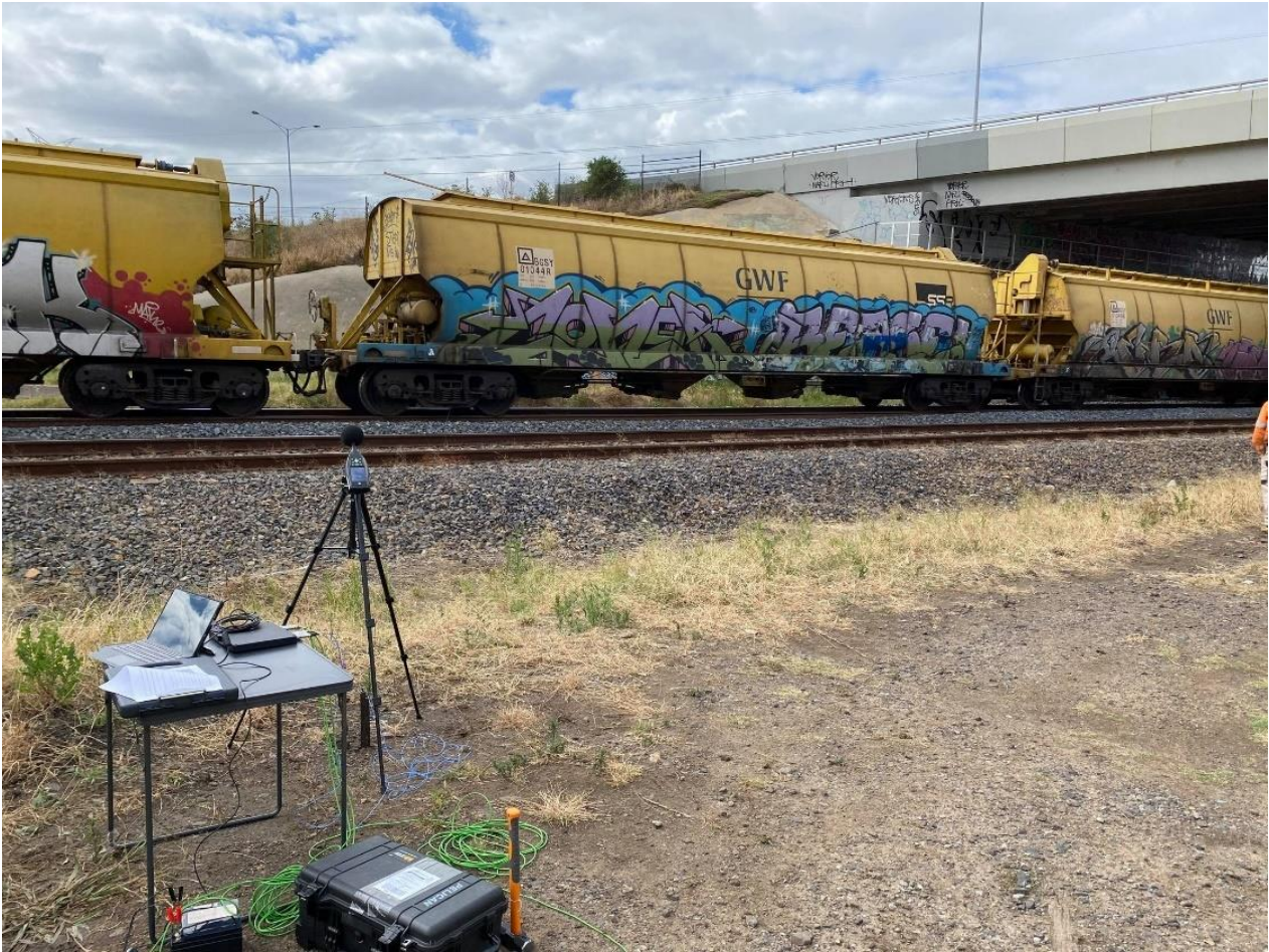
Figure 7-2 Vibration measurement equipment setup for measurement of rail pass-bys along Albion-Jacana link in December 2020
