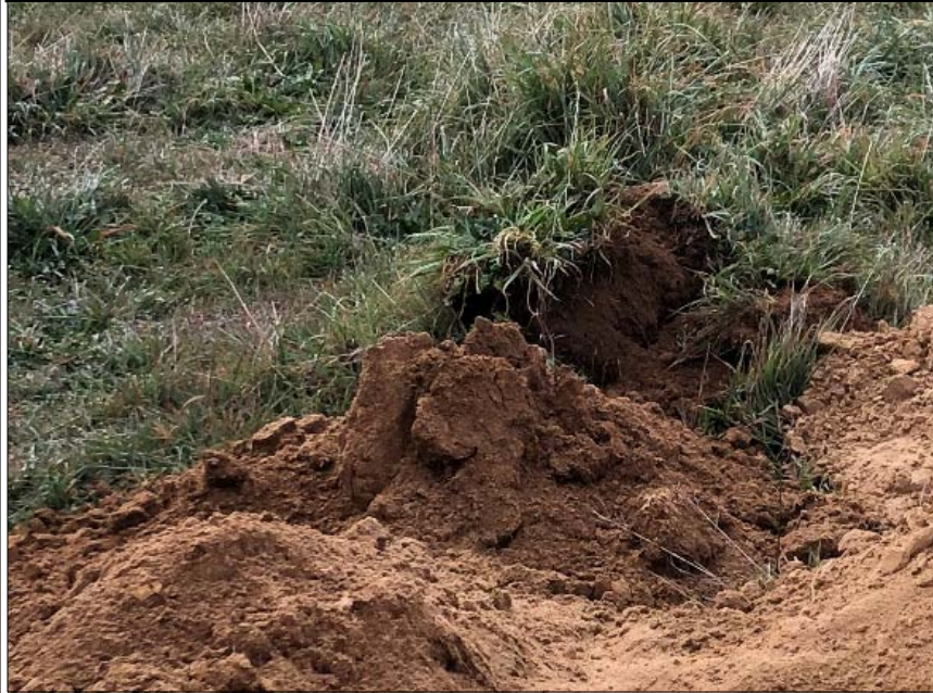
TP04 –VERY FINE VERY LOOSE SILT WITH SOME GRAVEL 0.9– 1.5 M
