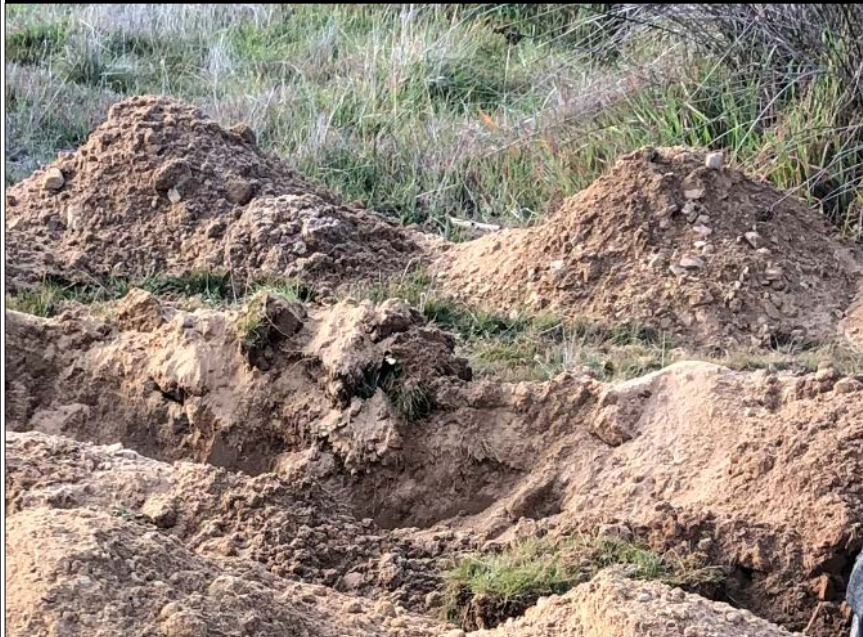
TP06 – VERY SOFT FINE SANDY SILT WITH GRAVEL 1.0 – 1.6 M
