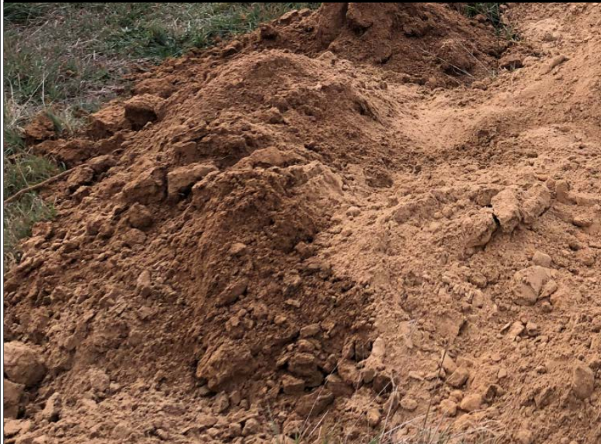
TP04 – BROWN LOOSE COARSE SILTY SAND 0.1 – 0.9 M
