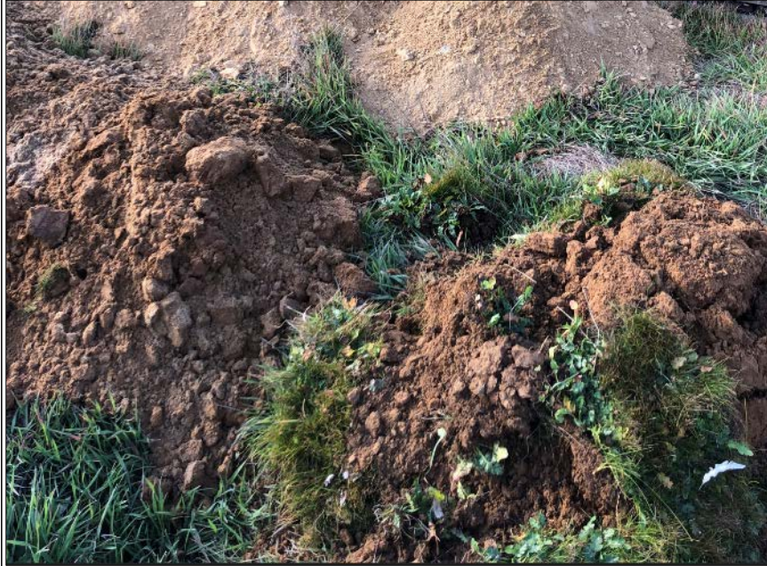
TP06 – VERY LOOSE FINE SOFT SILT 1.6 – 2.5 M
