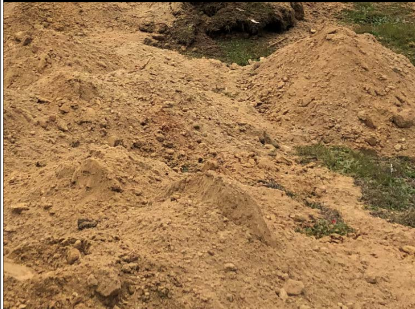
TP02 – LIGHTER VERY LOOSE SOFT SANDY SILT 1.1 – 1.8 M
