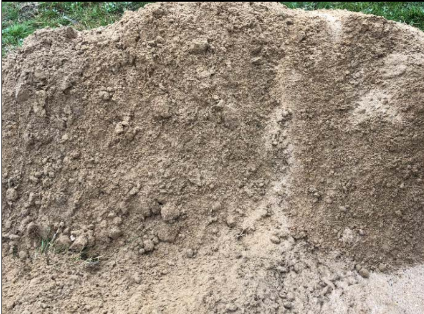
TP01 – VERY LOOSE SOFT AND FINE SANDY SILT 0.5 – 1.6 M
