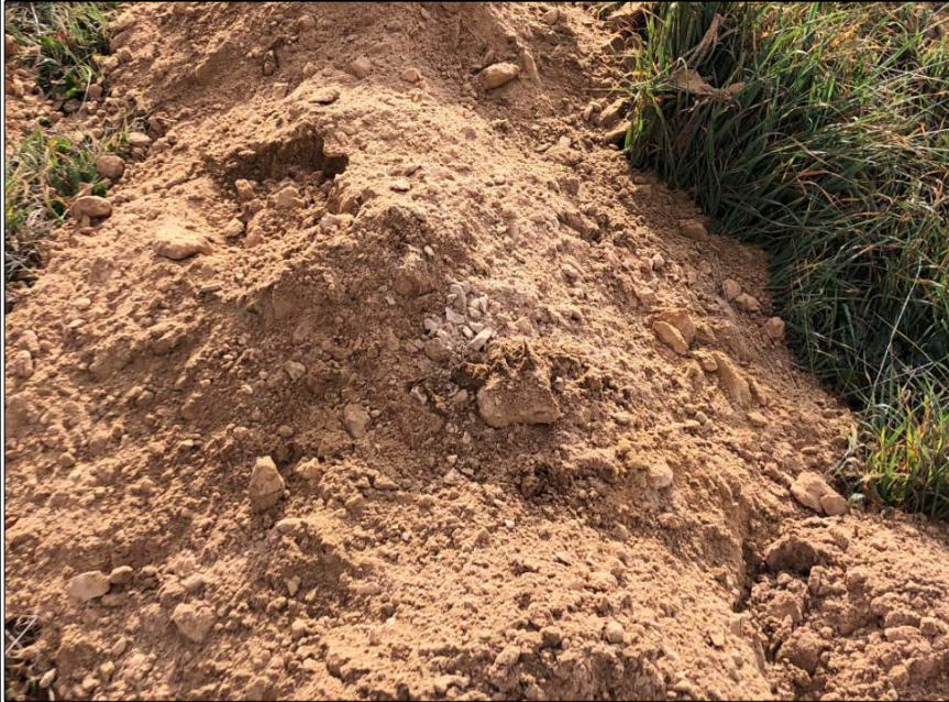
TP04 – NATURAL MATERIAL – ORANGE/RED SANDY SILT WITH CLAYEY CLUMPS 2.1 M
