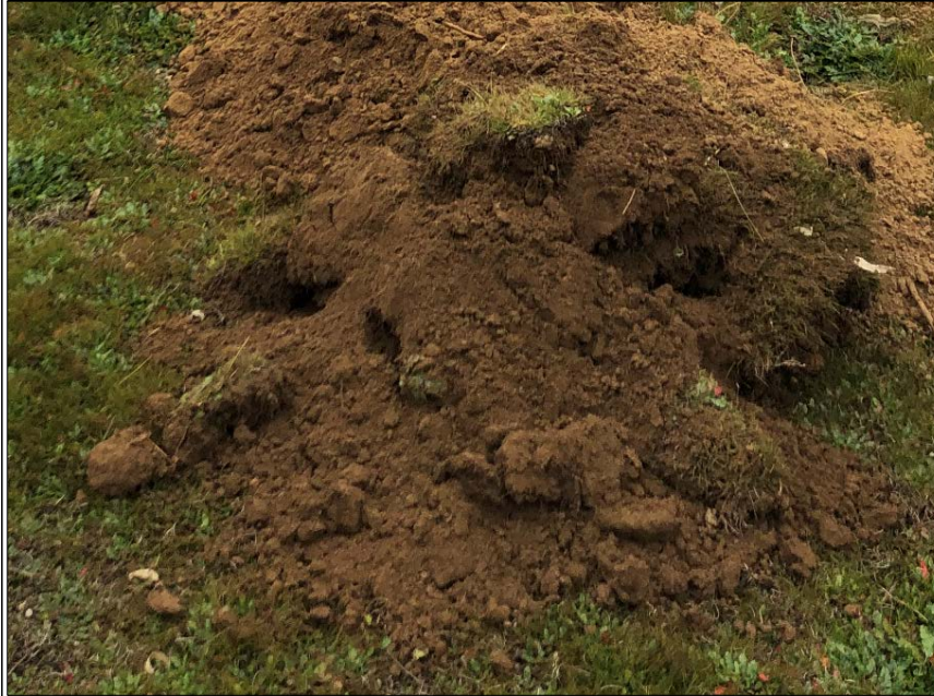
TP02 – LIGHTER VERY LOOSE SOFT SANDY SILT 1.1 – 1.8 M
