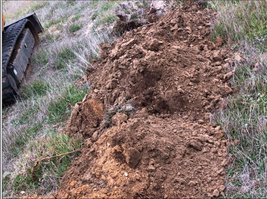
TP03 – FINE VERY LOOSE SOFT SANDY SILT WITH LESS GRAVEL 1.6 – 2.0 M
