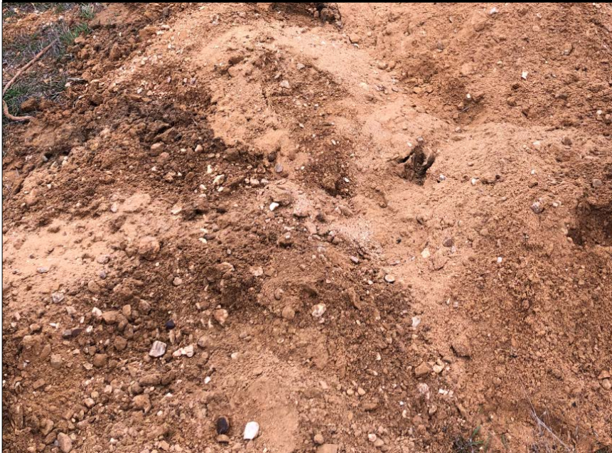
TP03 – LOOSE SOFT COARSE SILTY SAND WITH GRAVELS 0.4 – 1.6 M
