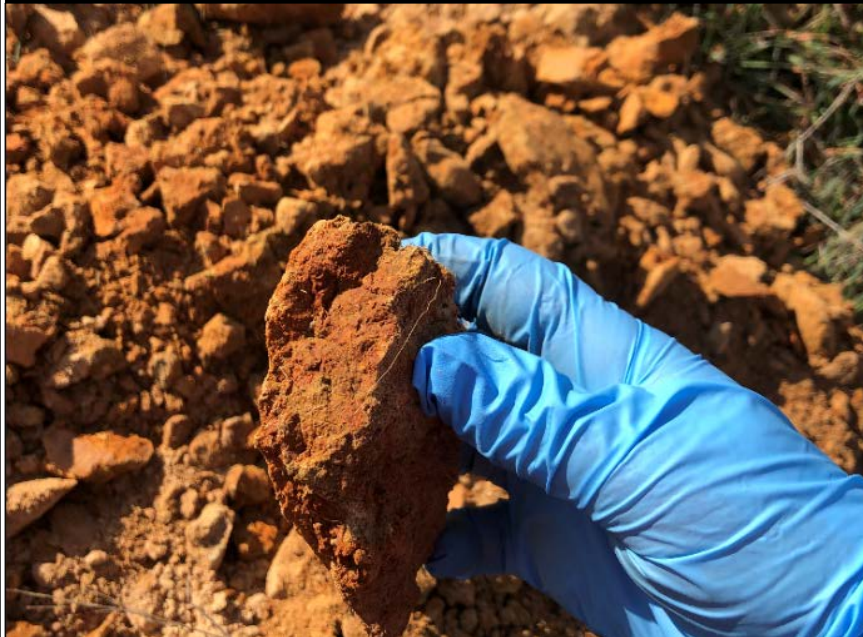
TP04 – NATURAL MATERIAL – ORANGE/RED SANDY SILT WITH CLAYEY CLUMPS 2.1 M
