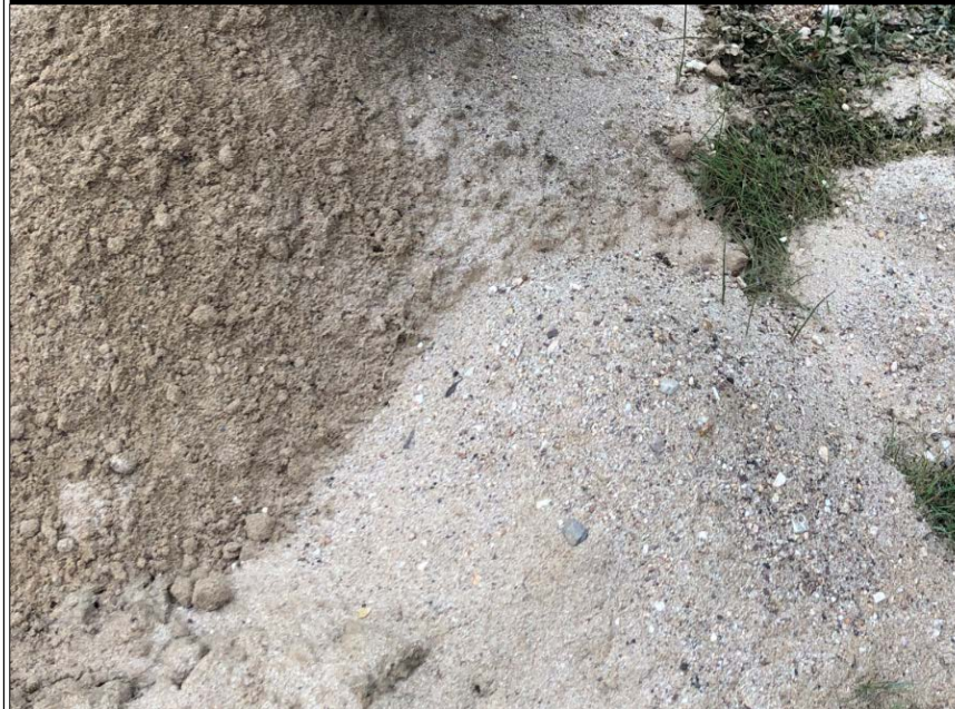
TP01 – LOOSE COARSE SAND WITH GRAVELLY LAYER BETWEEN 1.6 – 2 M
