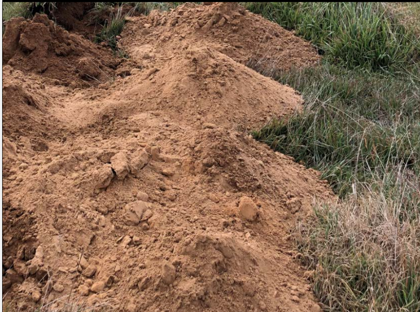
TP04 –VERY FINE VERY LOOSE SILT WITH SOME GRAVEL 0.9– 1.5 M
