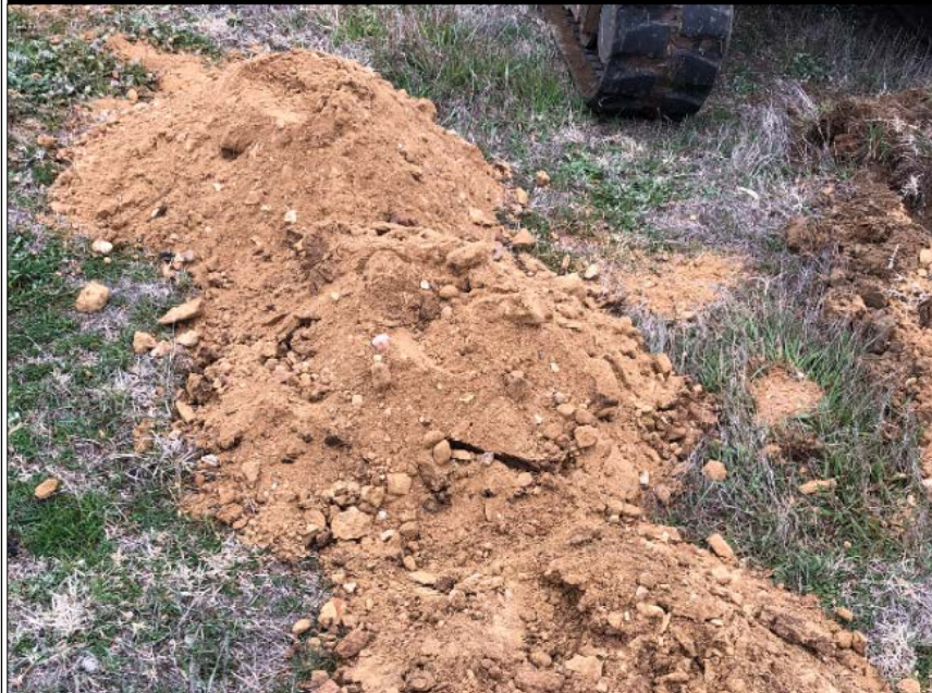
TP03 – FINE VERY LOOSE SOFT SANDY SILT WITH LESS GRAVEL 1.6 – 2.0 M
