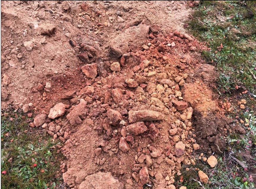
TP02 – NATURAL MATERIAL - RED/ORANGE SILTY SAND
