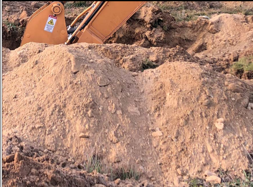
TP06 – VERY LOOSE FINE SOFT SILT 1.6 – 2.5 M
