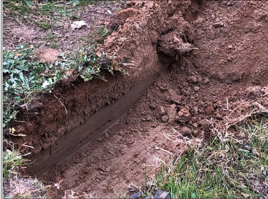
TP01 – LOOSE COARSE SAND WITH GRAVELLY LAYER BETWEEN 1.6 – 2 M
