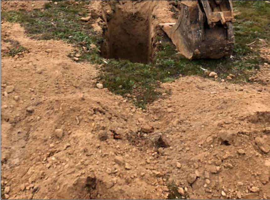
TP02 – LIGHTER VERY LOOSE SOFT SANDY SILT WITH GRAVEL LAYER 1.8 – 2.2 M
