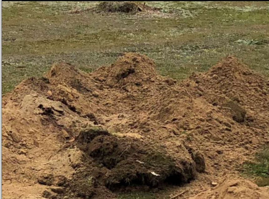
TP02 – LOOSE SOFT SILTY SAND 0.2 – 1.1 M
