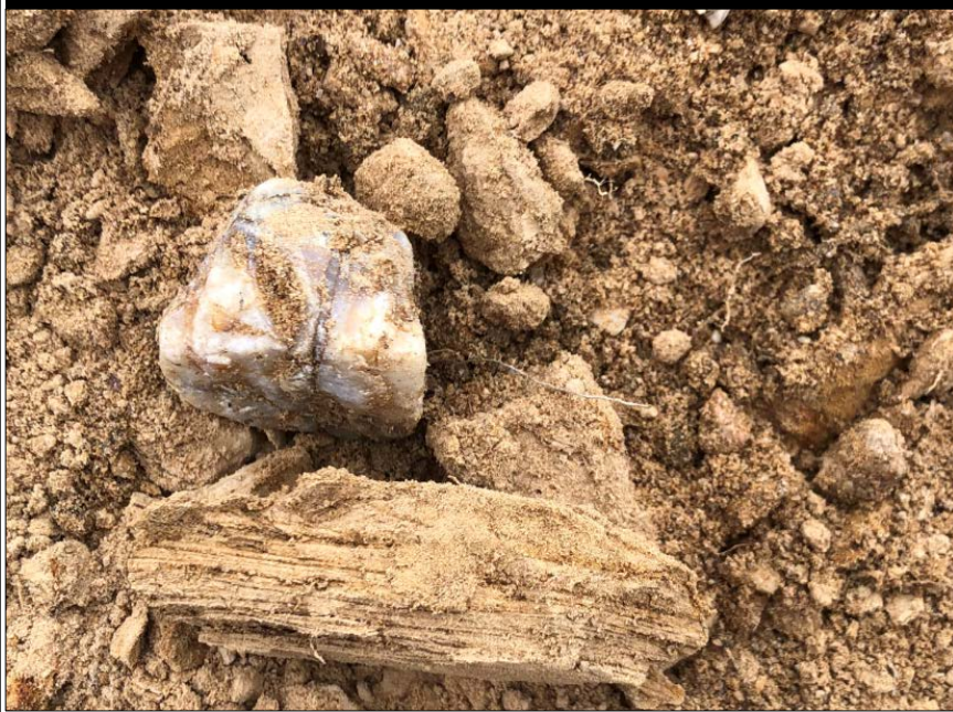
TP03 – QUARTZ AND LAYERED TAILINGS BETWEEN 0.4 – 1.6 M
