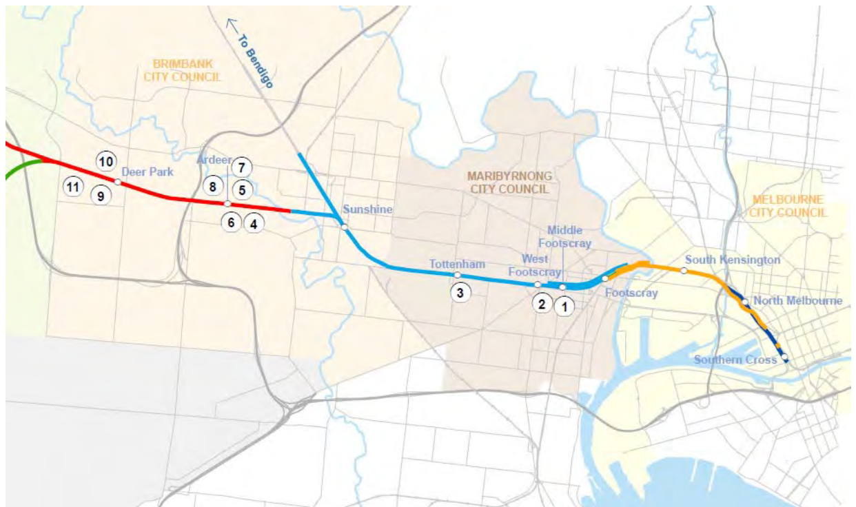
Figure 28 Location of predicted noise barriers to limit night-time noise to 60 dBL Aeq,9hr
