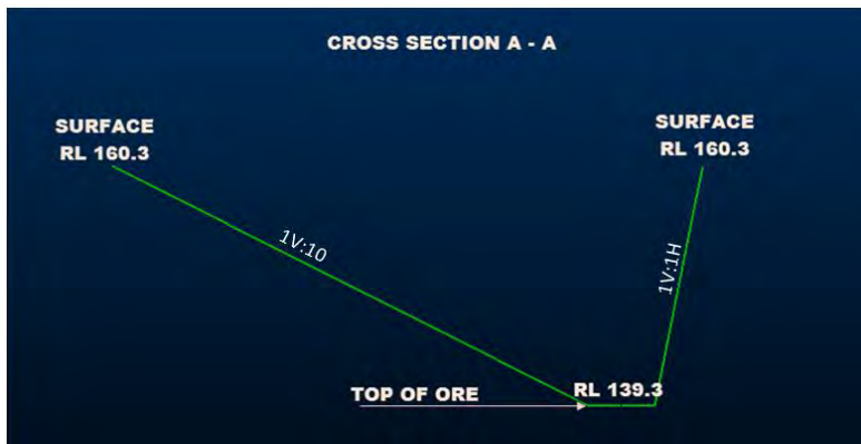
Figure 5-3 Cross section A-A at test pit (vertical exaggeration = 5.0)
