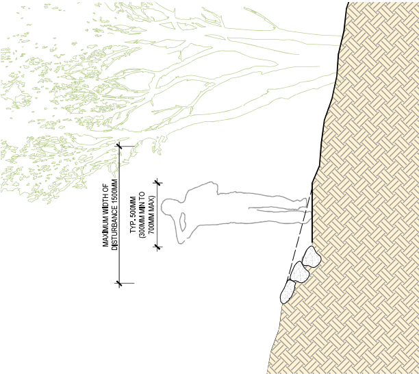
TYPICAL PATH CROSS SECTION - FULL BENCH 1:20
