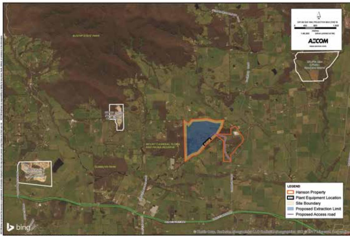
The key activities of the proposed quarry will include stripping of overburden, blasting of rock, haulage to a crushing and screening plant, stockpile storage of processed material and the transport offsite of purchased products. A key development activity will be the selection of the access road to the site.
