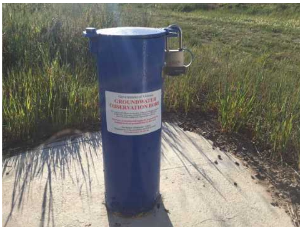
Figure 7 – Photo of Existing Groundwater Bore
