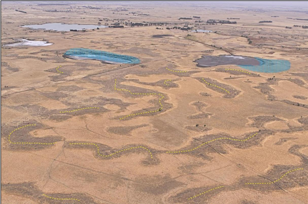
Figure 74. Part of geoscience Site 4 showing ridge crests possible cavern entrance sites (yellow line) and exclusion areas (blue shading).
