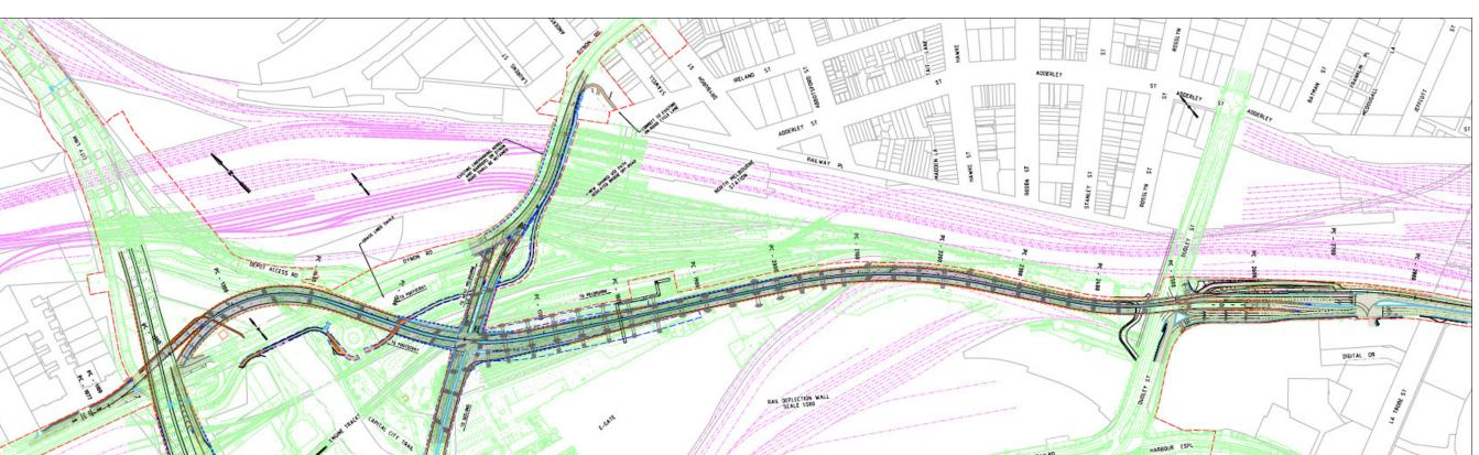
Figure 5-1 Plan view showing the horizontal alignment for the lowered Wurundjeri Way extension
