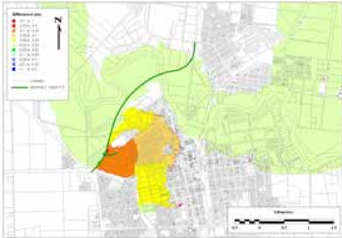
Figure 7-6 Flood difference for the preliminary Mid West 2 – Option 2.5 for the 5% AEP
