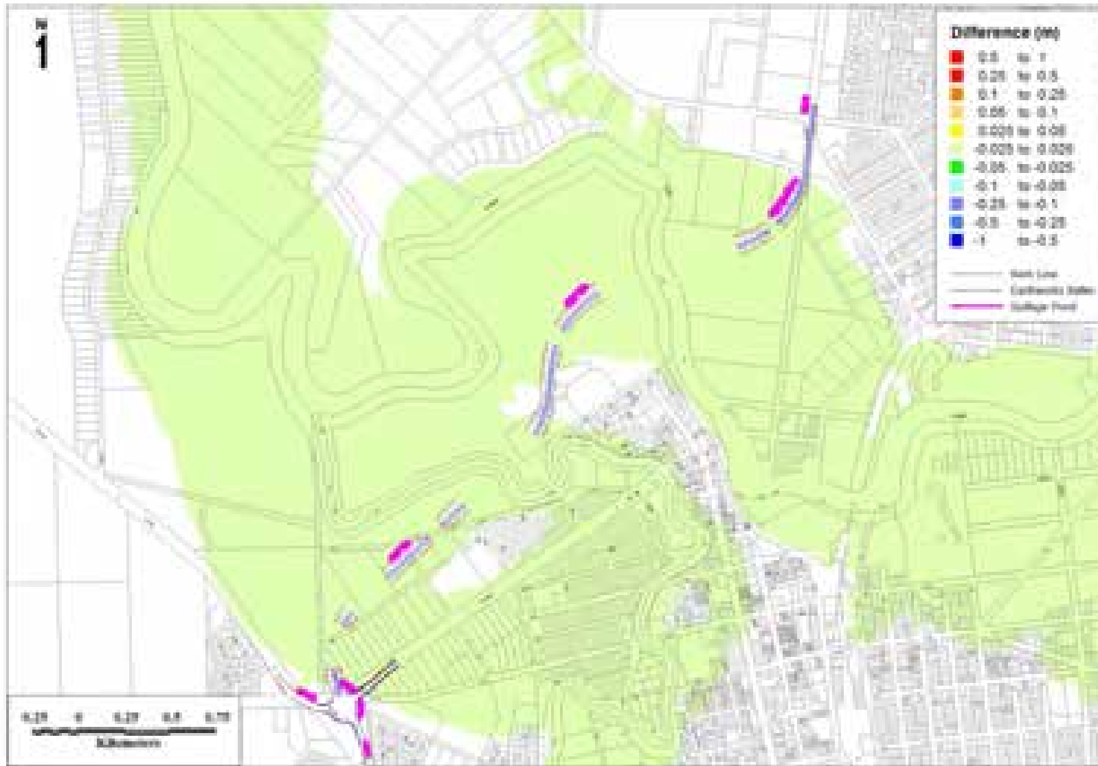
Figure 8-9 Alignment 2B peak flood height differences from existing for the 2% AEP
