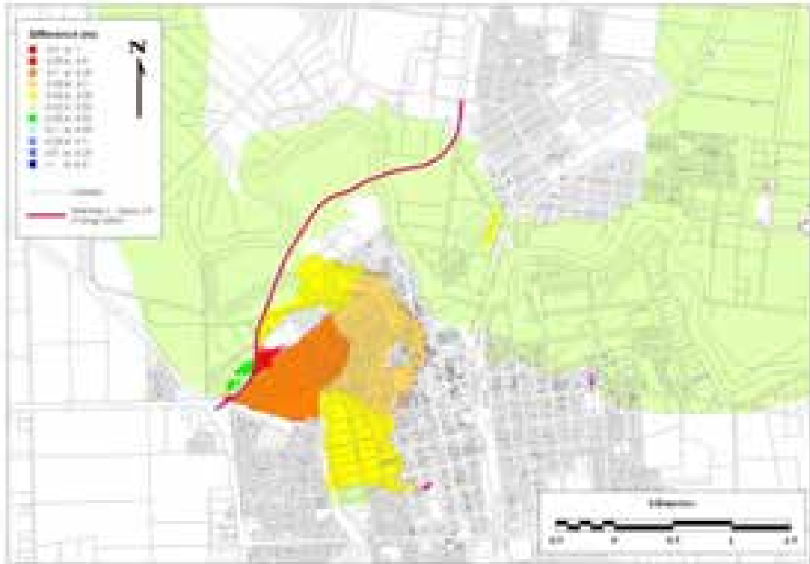
Figure 7-7 Flood difference for the preliminary Mid West 2 – Option 2.6 for the 5% AEP
