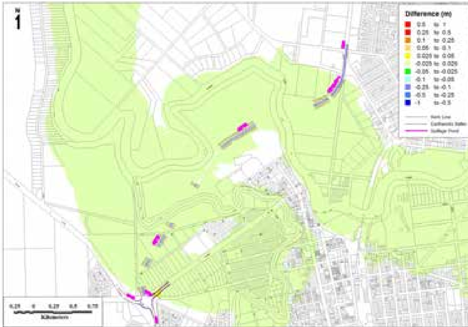
Figure 8-5 Alignment 2A peak flood height differences from existing for the 5% AEP
