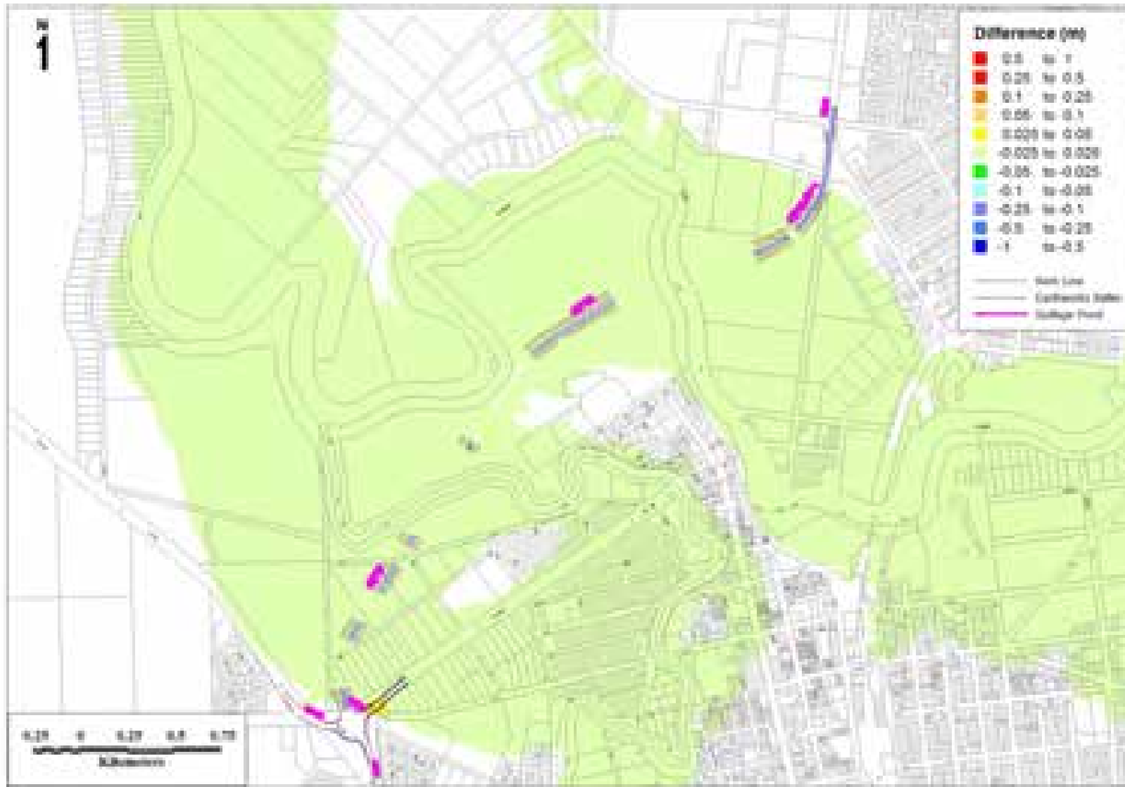
Figure 8-6 Alignment 2A peak flood height differences from existing for the 2% AEP
