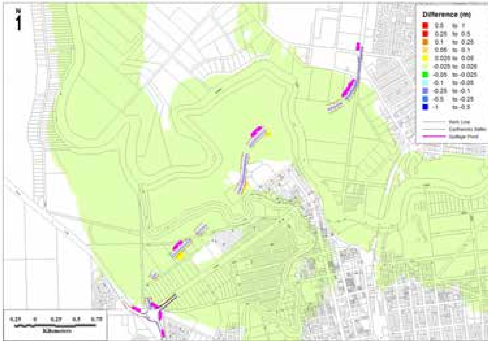
Figure 8-10 Alignment 2B peak flood height differences from existing for the 1% AEP
