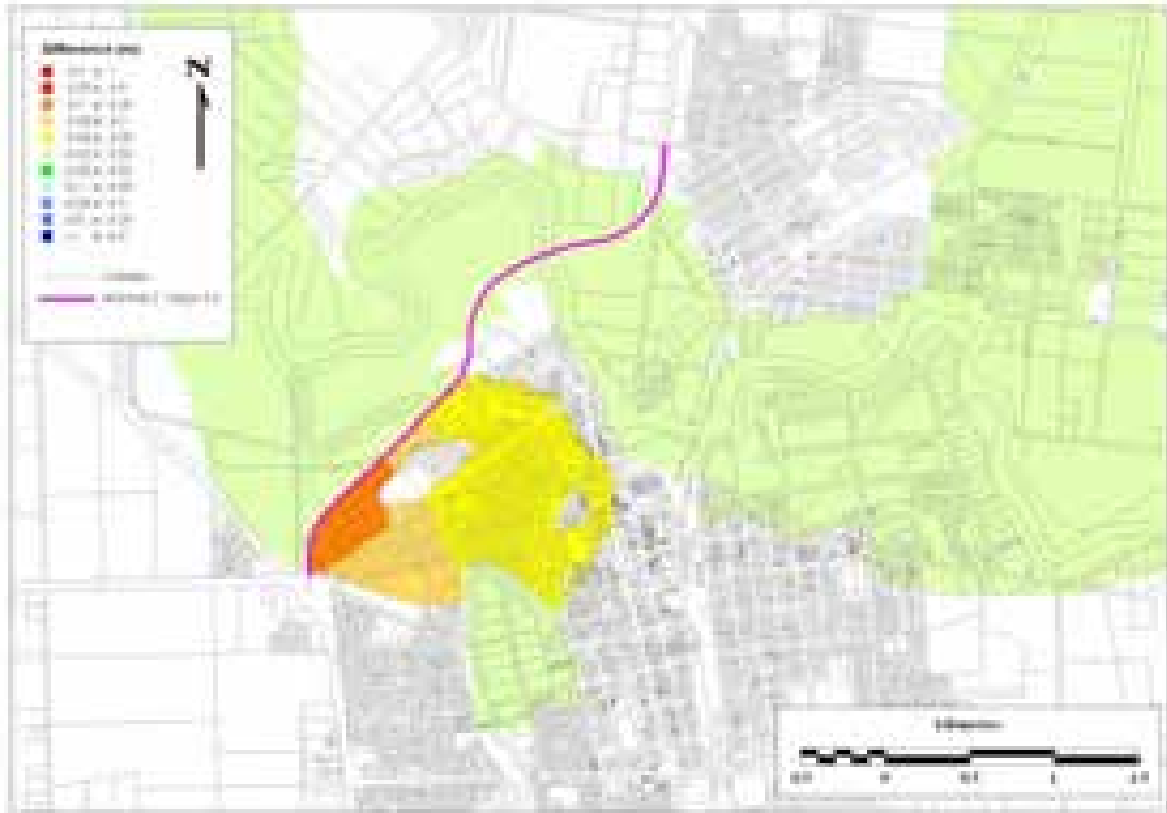
Figure 7-4 Flood difference for the preliminary Mid West 2 – Option 2.3 for the 5% AEP
