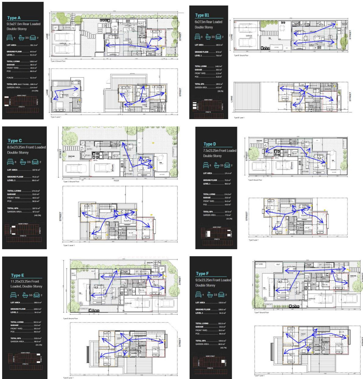
Figure 2: Breeze paths within the townhouses on ground and first floor. Type B2 has been left out as the floor designs is identical to Type B1.
