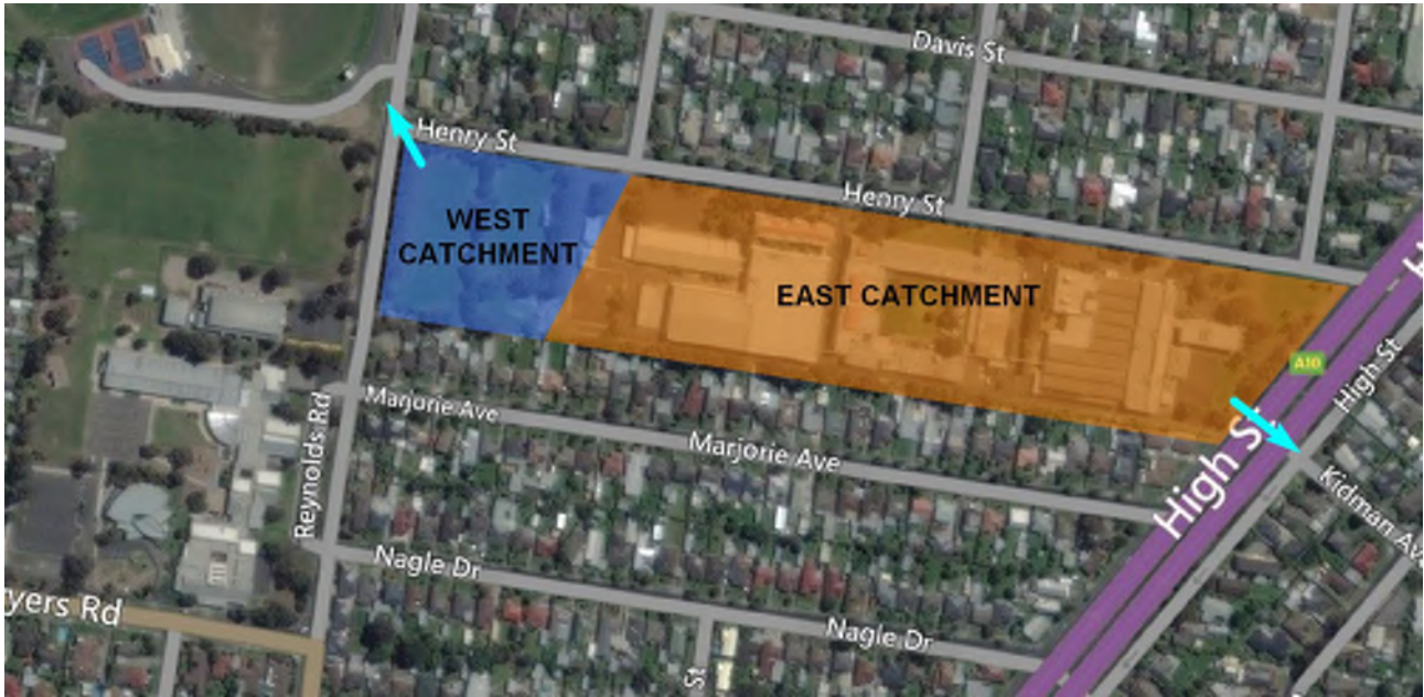
Figure 2.3: Internal sub-catchments & Discharge Locations
