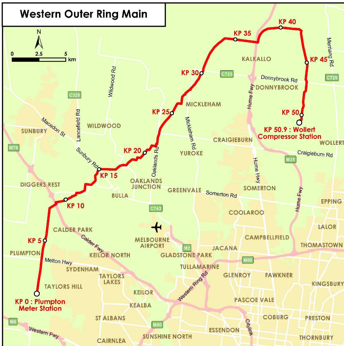
Figure 1: Proposed pipeline route (source: APA).
