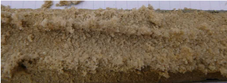
SPT Depth 4.5-4.95m, close up view
