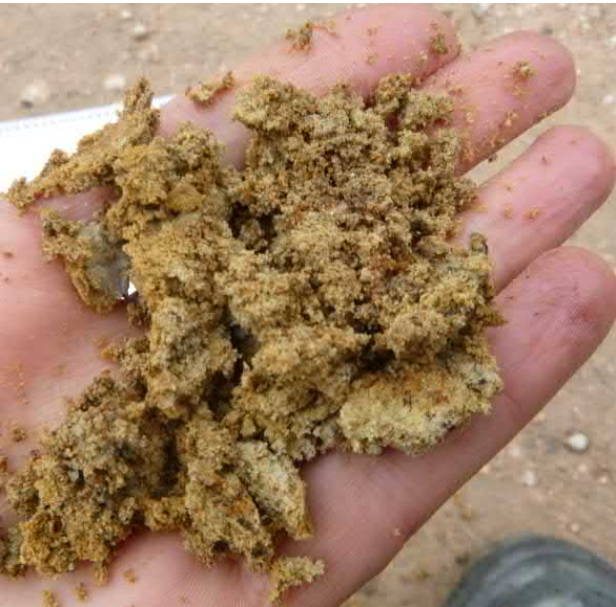
SPT Depth 3.0-3.45m, close up view
