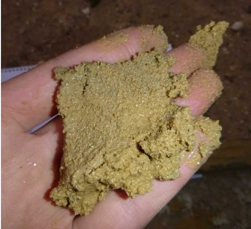
SPT Depth 6.0-6.45m, close up view
