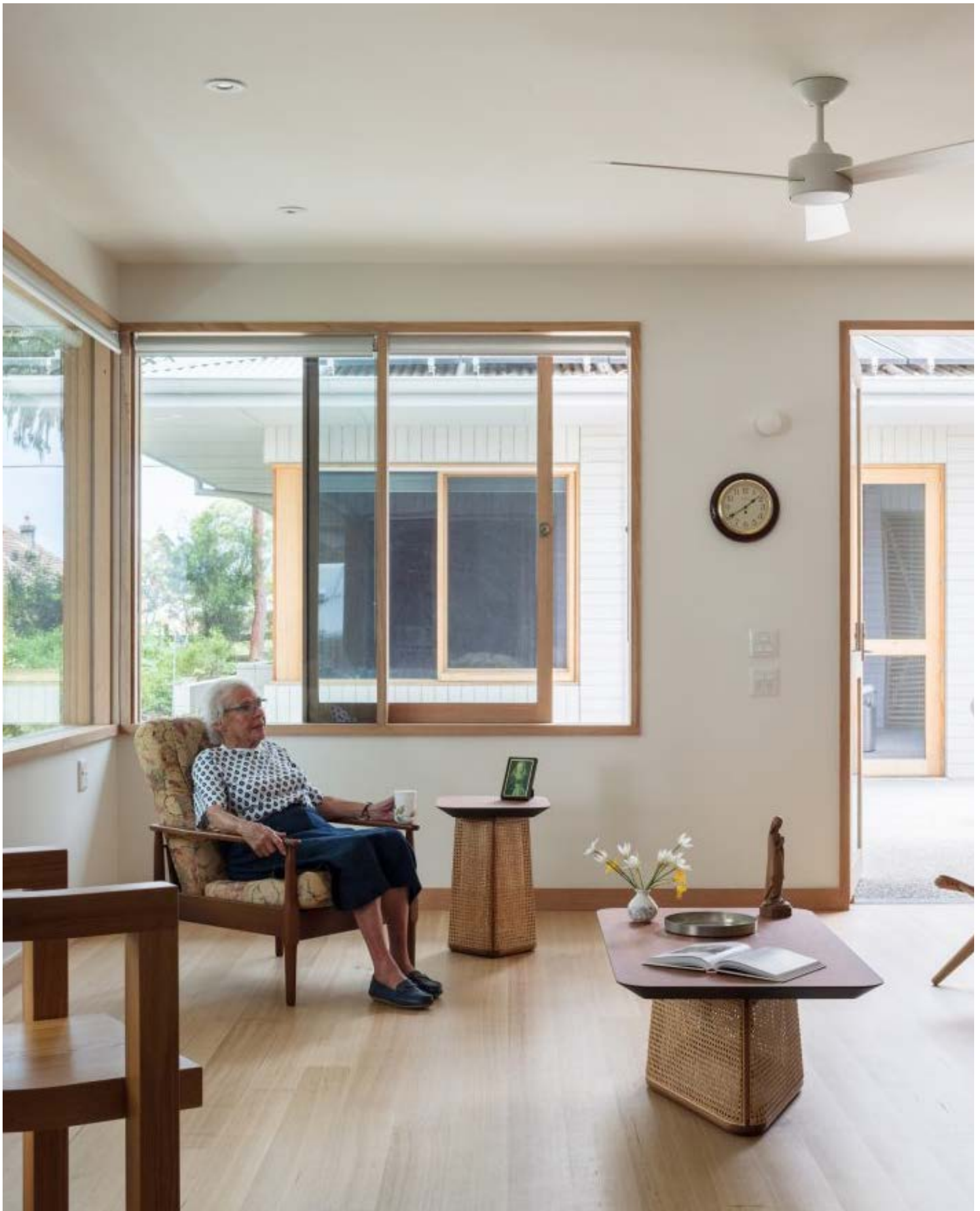
▲ Figure 72. Large sliding windows and doors allow occupants to maximise natural ventilation which can create a healthier indoor environment.
