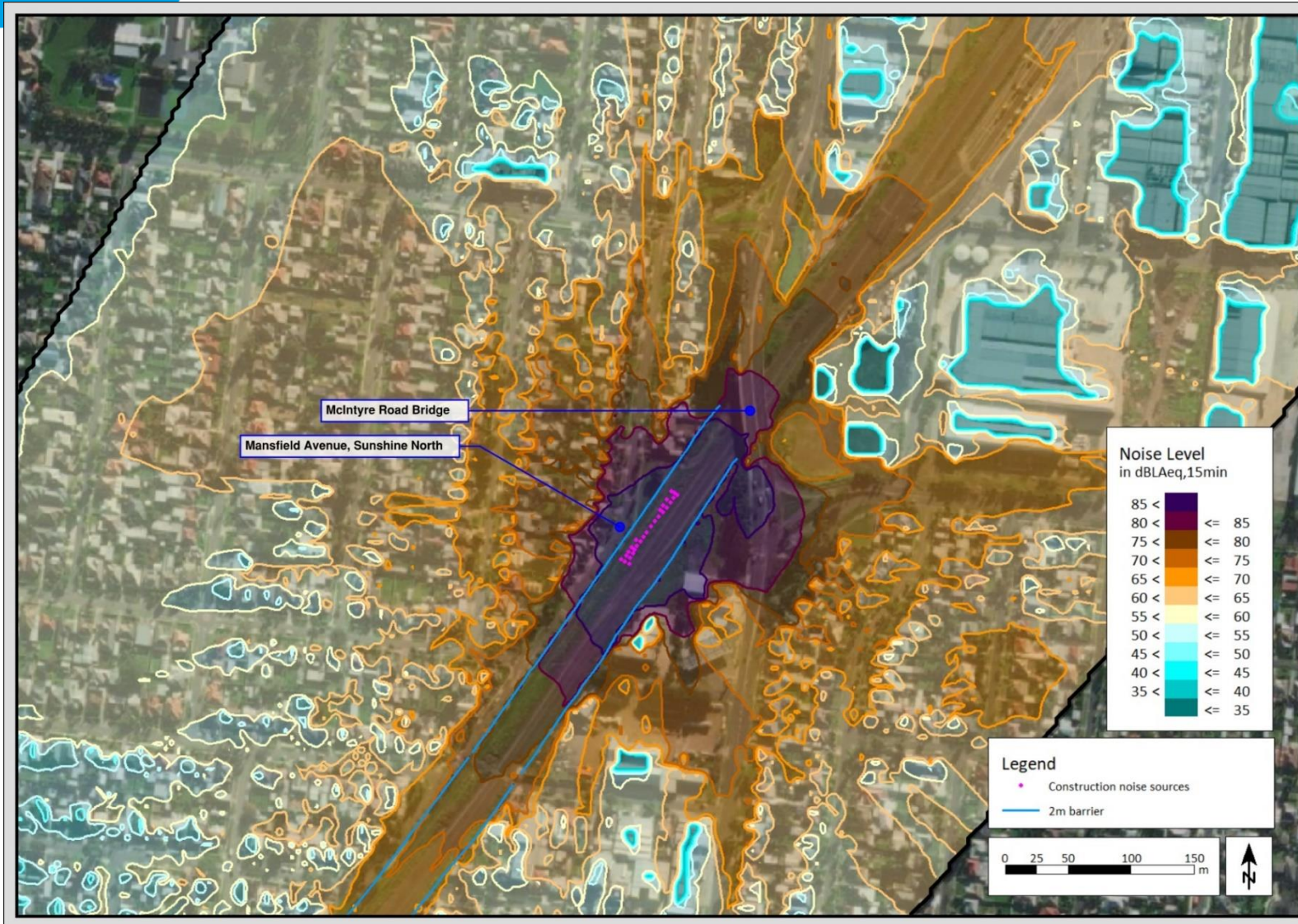
Figure A.28 Predicted construction noise levels for Scenario 10 – ACP Track formation works with 2 m high noise barriers (north)
