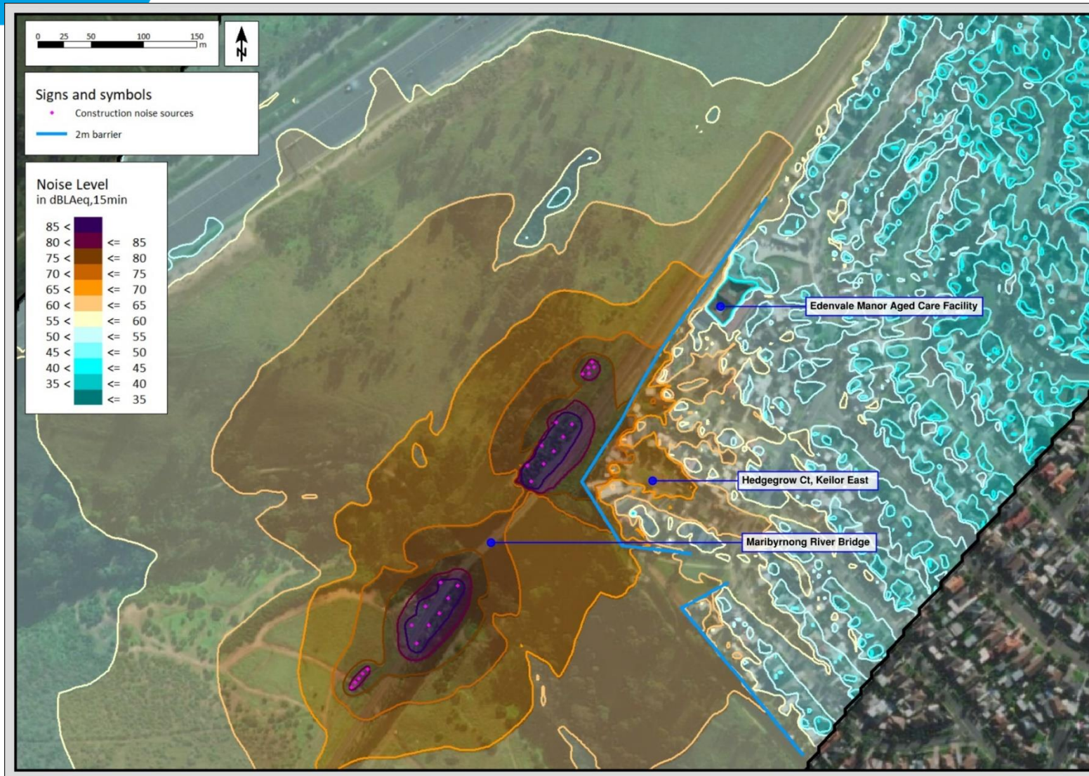
Figure A.32 Predicted construction noise levels for Scenario 14 - MAR Maribyrnong River Bridge Tower Mobilisation with 2 m high noise barriers
