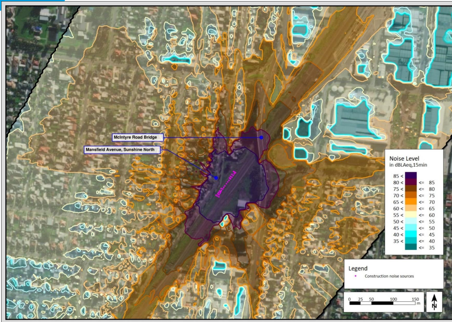
Figure A.13 Predicted construction noise levels for Scenario 10 - ACP Track formation works (north)
