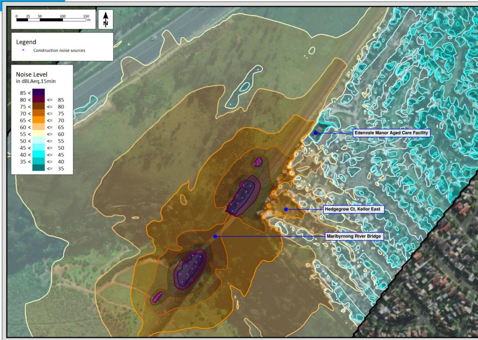
Figure A.17 Predicted construction noise levels for Scenario 14 - Maribyrnong River Bridge Tower Mobilisation
