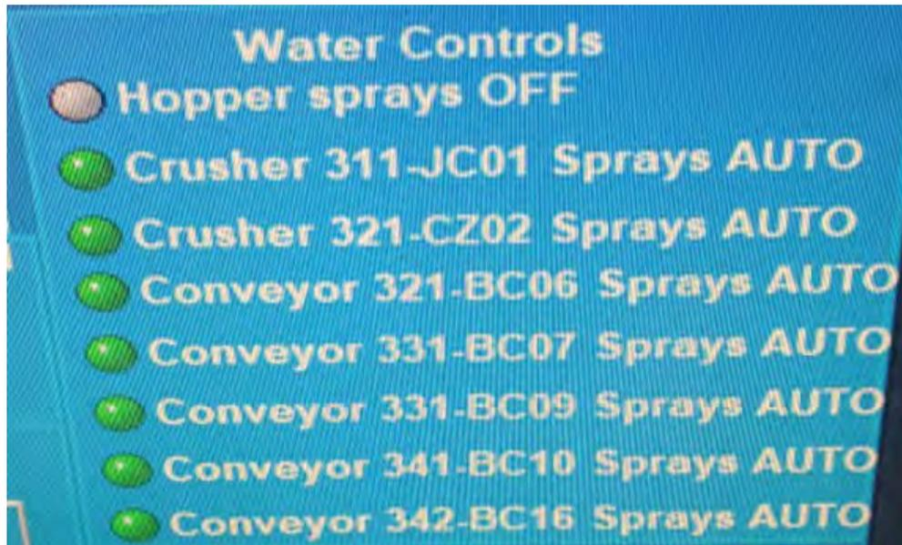
When the sprays are activated in 'AUTO', they will turn on and off automatically depending on the % load on the conveyor or crusher so as not to over/under supply the water. This must be the standard mode of operation.
