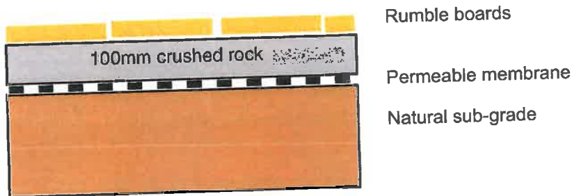
Diagram 2 Indicative ground protection system - adapted from AS4970 Clause 4.5.3 Ground protection.
