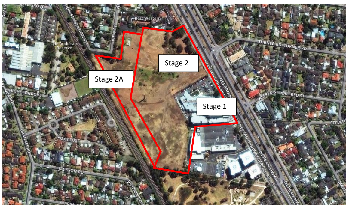
Figure 6 - Staging Areas for site remediation
