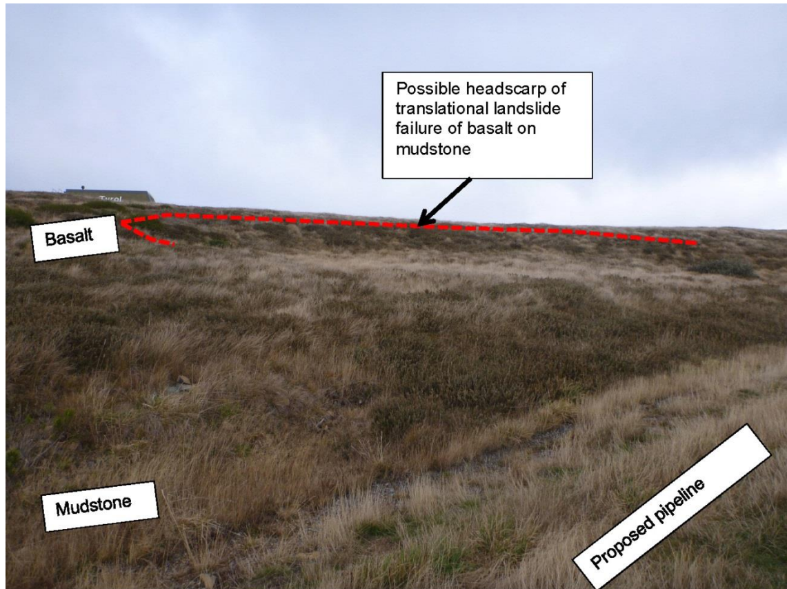
Plate 5. Possible area of instability to south of main pipeline alignment.
